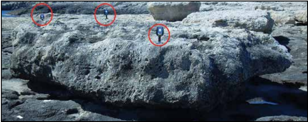
Fig. 5. Megaboulder scanned on the coastal area of Augusta (Southern Italy). Red circles highlighted the rectangular targets used to co-registrate all the TLS scan.
