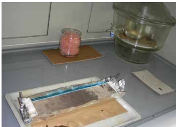
Fig. 6. Impregnation of the soft core sediment to get a hardened sample for the preparation of a thin section (from Srisutam & Wagner, 2010c)
