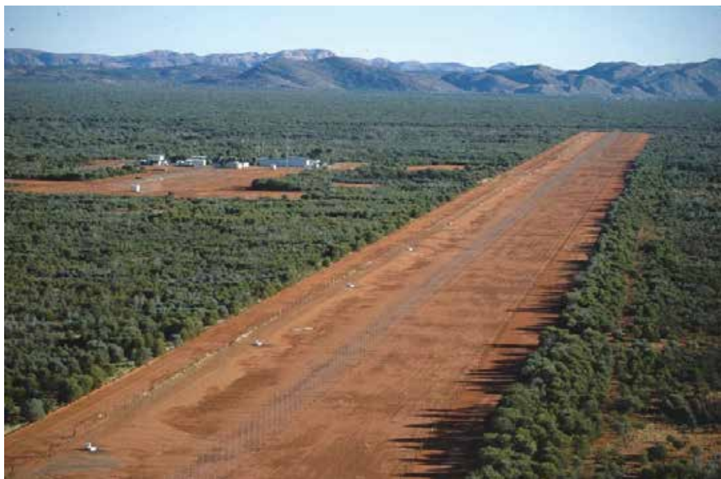
Fig. 2. Aerial view of the 2.8 km receiving array of the Australian Jindalee skywave radar, operational since 1982.
