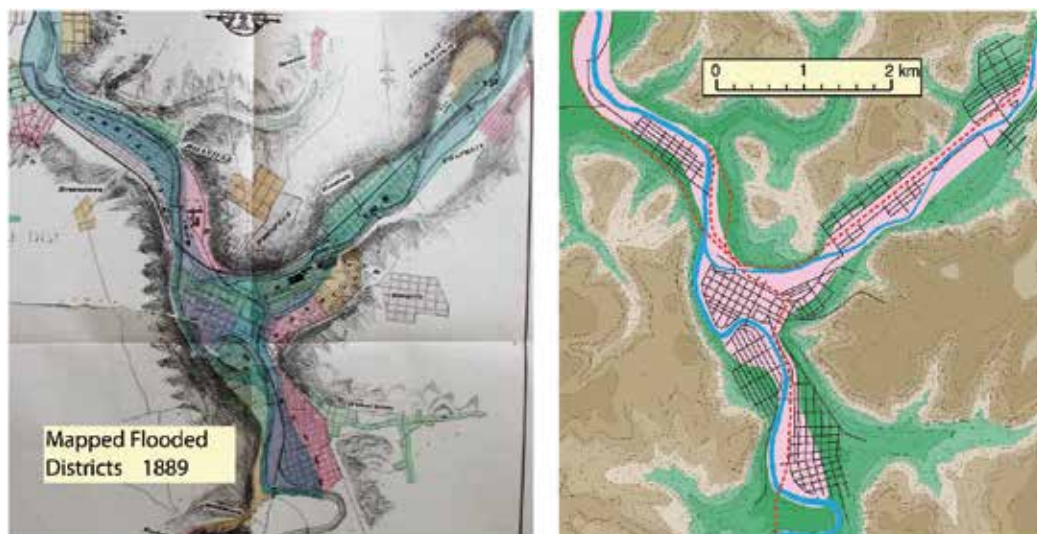
Fig. 4. (Left) Plate from Cadwell's 1890 Atlas of Cambria County. Bluish-green tint covers the "flooded districts" of the Conemaugh Valley. (Right) My translation of Cadwell's flood zone over today's topography and a 1900 street map. Ideally, the simulated flood will cover the pink area. Dashed red lines are railroads.
