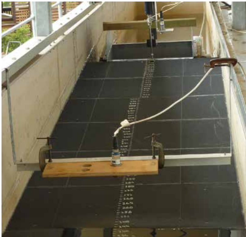
Fig. 4. Photo of upper beach panels, overtopping tank and instrumentation.
