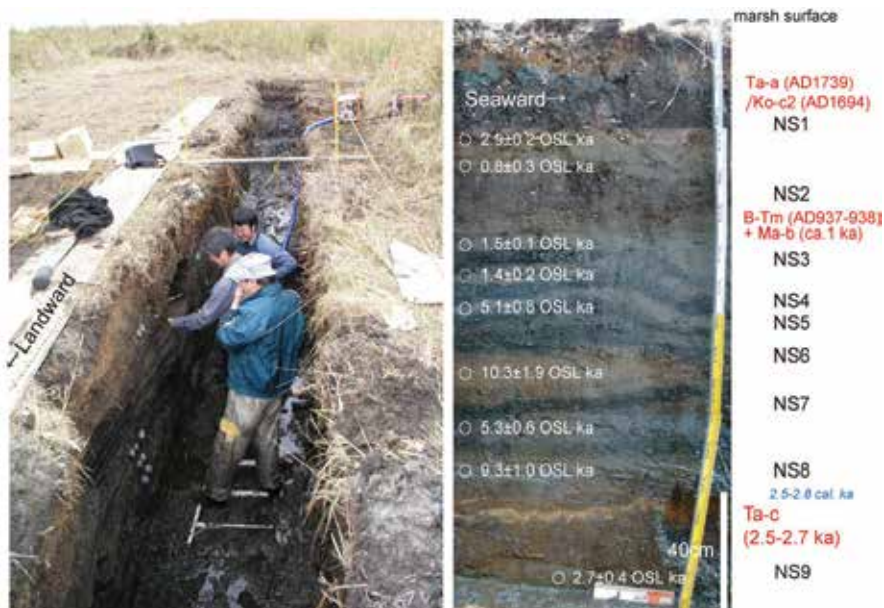
Fig. 6. Collection of samples for OSL dating at Shig trench (left). Photograph of the trench wall showing the OSL sampling horizons and dating results (right). AMS 14 C dating results, tephra layers and dates, and sand beds NS1 to NS9 are indicated to the right of the photograph.
