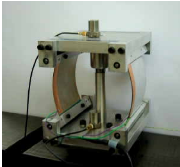
Fig. 10. ATVA with variable-curvature piezo-actuated beams (Bonello et al., 2005)
