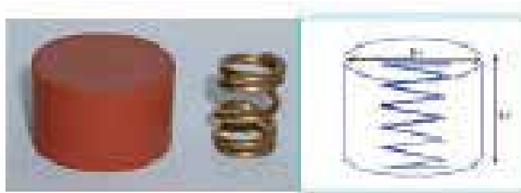
Fig. 17. Example of Composite Rubber/SMA spring damper
