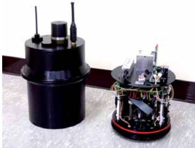
Fig. 3. Electronics system of P-SURO AUV.
