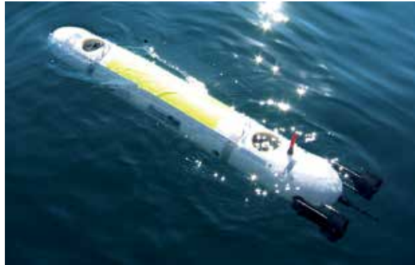
Fig. 1. Autonomous Underwater Vehicle MARES.
