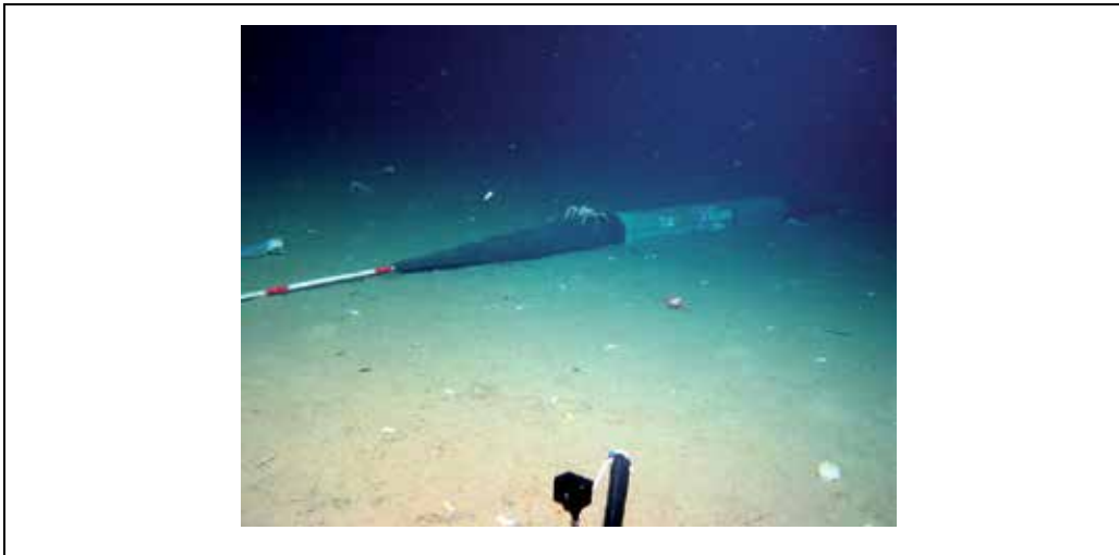
Fig. 3. In-lined cabled bottom pressure sensor deployed in the ocean.
