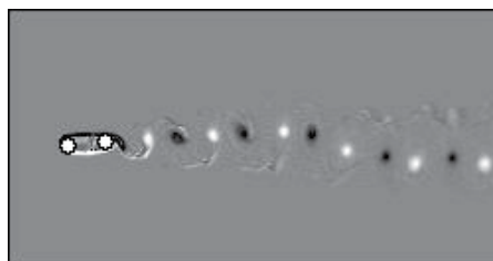
Fig. 8. Instantaneous vorticity field for L/D=2 and Re=39,500 .
