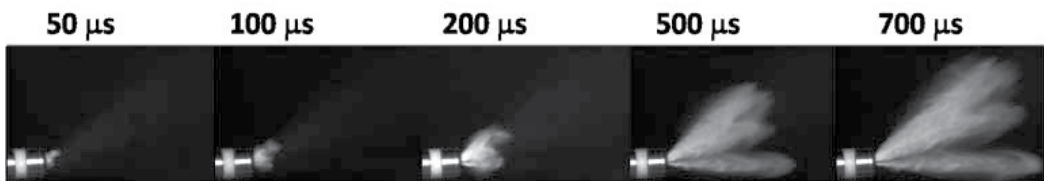
Fig. 6. Sequence of sprays from Injector #3 taken at different time from the SOI at P_{inj} = 10 \text{ MPa} , m_f = 50 \text{ mg} .
