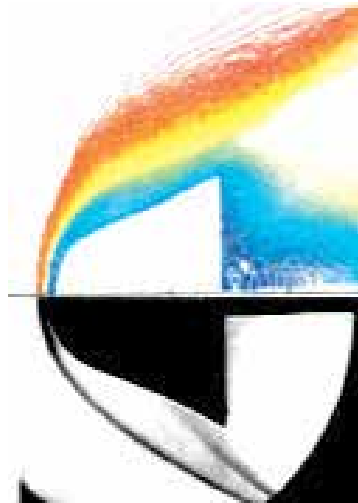
Fig. 4. Comparison between density contour and schlieren picture.
