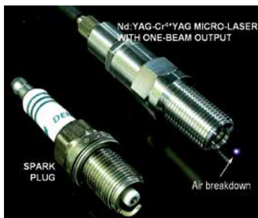
Fig. 9. Nd:YAG-Cr 4+ :YAG laser with one-beam output. Nd:YAG gain medium and Cr 4+ :YAG SA were single crystals; all optical components (including the output mirror) were discrete elements. Air breakdown is shown and size comparison is made with a spark plug.
