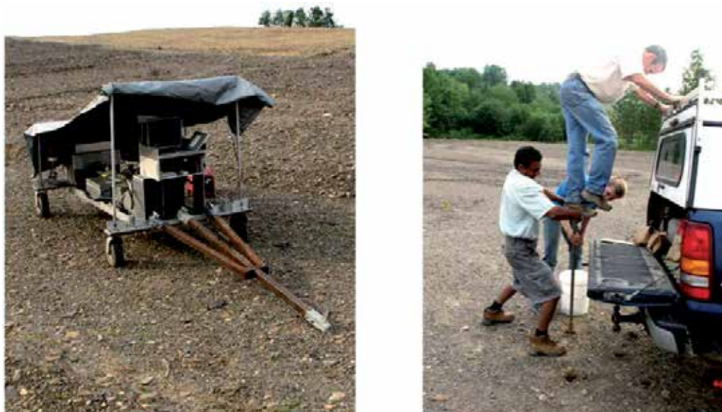
Fig. 14. Comparison of sampling abandoned minefield restored with its original overburden using the INS system on the left, and an attempt using conventional coring on the right, many cores could not be sampled deeper than 10 cm.
