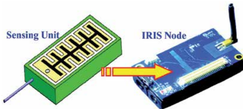
Fig. 23. Self-powered wireless corrosion monitoring sensor
