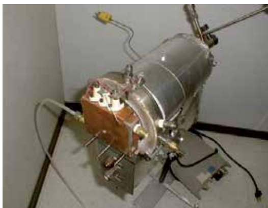
Fig. 4. Photograph of a silicon concentrator solar cell based TPV prototype system (Qiu & Hayden, 2006).
