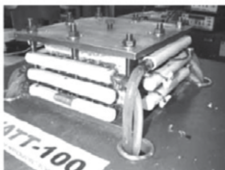
Fig. 3. Photograph of a thermoelectric power generator produced by the Japanese Energy Conservation Center, which used waste heat as energy source to generate an electric power density of 100 kW/m 3 (Weiling & Shantung, 2004).
