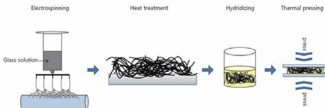
Fig. 11. Schematic illustration of the processing introduced to fabricate bioactive glass nanofiber and its nanocomposite result with PLA.
