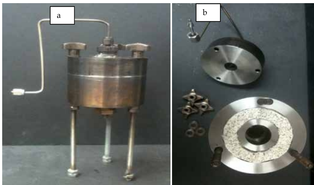
Fig. 16. (a) Reactor (b) Internal view of the reactor and screws.
