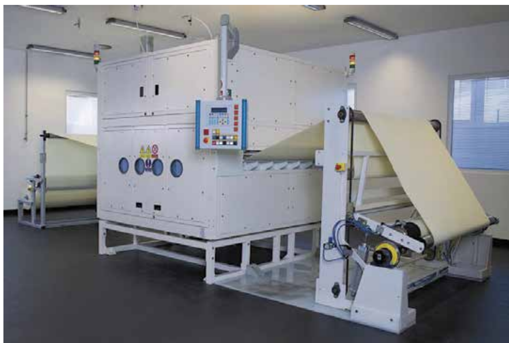
Fig. 10. Nozzle-less production electrospinning line (Nanospider™).
