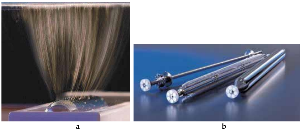
Fig. 7. Free liquid surface electrospinning from a rotating electrode (a) and various types of spinning electrodes (b).
