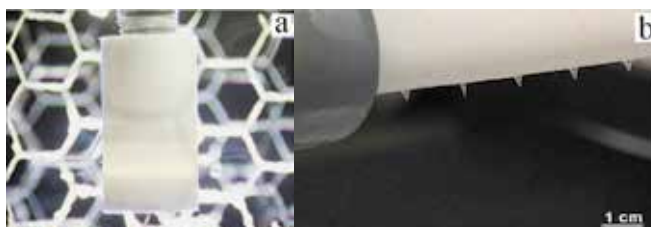
Fig. 3. (a) Electrospinning using a vertical tubular foam spinneret (Dosunmu et al. , 2006), (b) horizontal tube electrospinning (Varabhas et al. , 2008).
