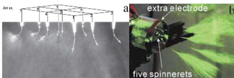
Fig. 2. (a) A multi-jet electrospinning setup (Theron et al. , 2005), (b) multi-jet electrospinning with a cylindrical auxiliary electrode (Kim et al. , 2006).
