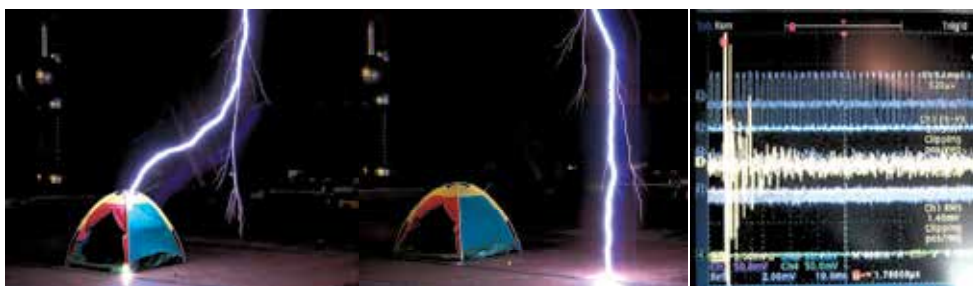
Fig. 15. Left : Basic structure of the tent as a model for the Faraday cage. There can be arcing if some metal is present inside the tent (no lightning safety), Mid : Lightning event occurs near the object due to slight moment of the electrode. Right : The measured electric field due to arcing (impact) of the lightning discharge on the model of Faraday cage.
