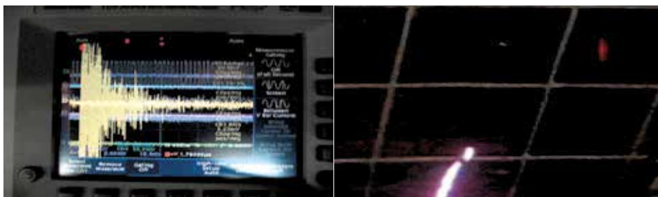
Fig. 14. Left : Lightning electric field captured with oscilloscope. A round-trip-time (direct and reflected) wave indicates many reflections from all walls of the chamber. The captured image shows similarities with natural lightning signal shown in Figure 20, Right : The striking phenomenon, upward lightning initiated by sharp objects in the vicinity of chamber ground was observed. In principle, this phenomenon occurs with sharp endings tall buildings like church etc. It has similarity with return stroke (RS) phenomenon.
