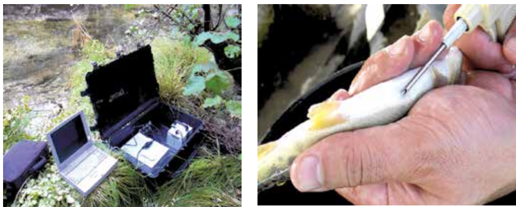
Fig. 5. PIT equipment (battery-pack and multi-point decoder- MPD) unit and PIT tagging procedures.
