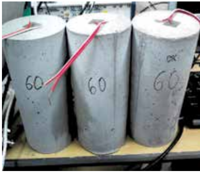
(a) 60MPa Concrete specimen
