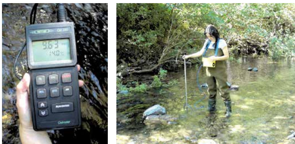
Fig. 4. Measuring temperature (°C) and water column velocity (m.s -1 ) in the Baceiro River (summer 2005).
