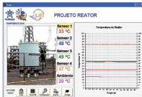
Fig. 3.1.8. Control software screen showing the graph of the four temperatures as well as the ambient temperature.
