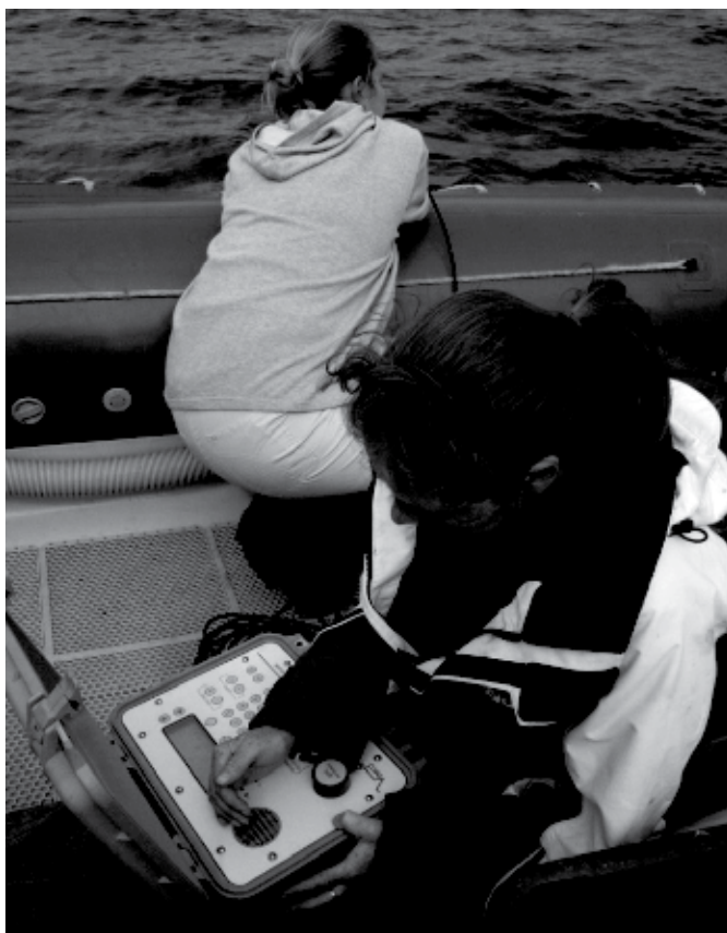
Fig. 11. Active tracking using a VH110 directional hydrophone, held in the water, and a VR100 receiver
