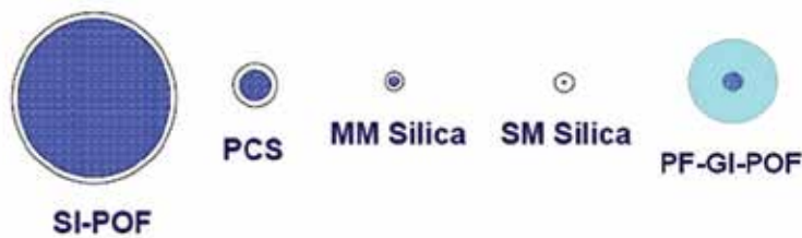
Fig. 2.1. Relative comparison of diameters in different kinds of fibers. SI-POF=step-index polymeric optical fiber; PCS=plastic cladding silica fiber; MM Silica=multimode silica fiber; SM silica=single mode silica fiber; PF-GI-POF=perfluorinated graded-index POF. The light color represents the cladding and dark color the core.
