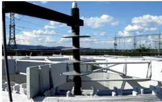
Fig. 3.1.6. One of the four sensors installed on the top of the coil.
