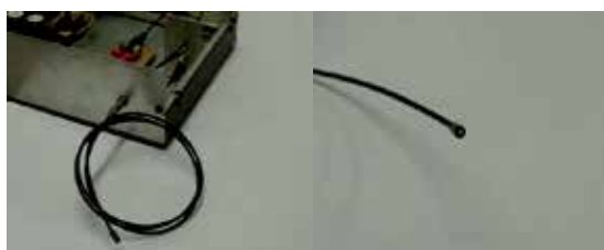
Fig. 3.1.2. Picture of the miniaturised POF-probe with hemispherical ruby crystal.
