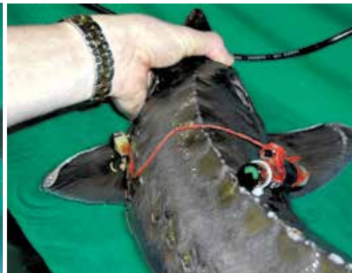
Fig. 48. Tag attached to right pectoral fin and connected to sensor situated on the left pectoral fin.
