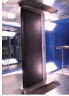
Fig. 52. Morphing wing system in the wind tunnel test runs
