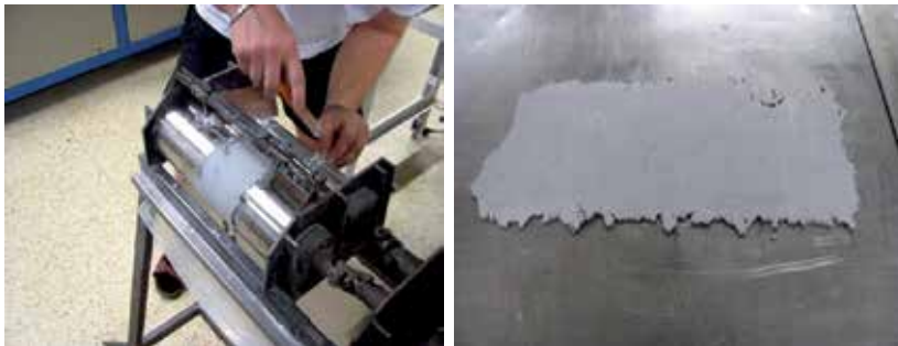
Figure 30. Preparation of strontium aluminate based MDF using twin roll mixer.
