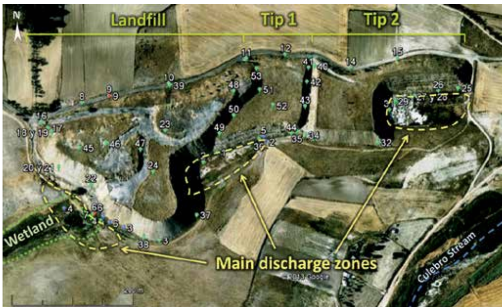
Figure 3. Main areas of the landfill and sites where capping soil samples were collected. 03/08/2009 Google Earth Image. UTM coordinates: X=442599 Y=4459459, 30T.
