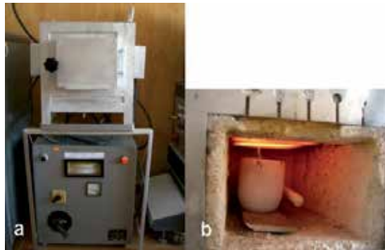
Figure 4. Plant biomass incineration: (a) heat treatment oven with forced rod, (b) incineration process
