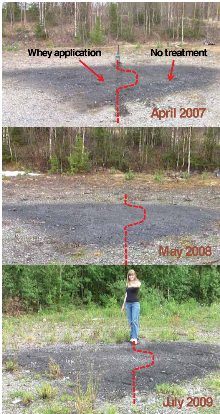
Figure 11. One time treatment of left part of oil spot with 200 l fresh milk whey.
