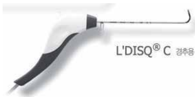
Figure 6. The wand and navigable tip of the L'DISQ-C is shown. The tip of the wand can be curved to the desired angle by rotating the control wheel. After placing the tip into the posterior annulus, plasma energy induced by radio-frequency is used to ablate and decompress the disc herniation.
