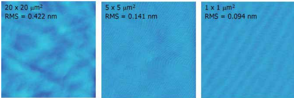
Figure 17. Microscopic surface morphology using AFM on GaN p-i-n structure grown on GaN/Sapphire template. No specific surface defects are observed [27]
