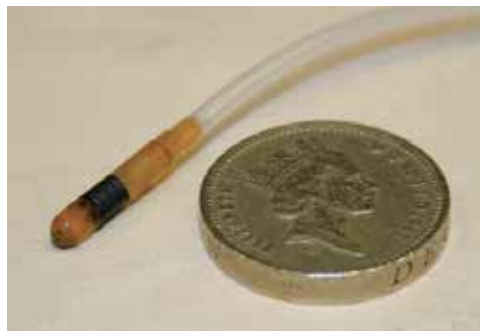
Figure 11. Ablation catheter with force sensor (Reference [29]). The outer diameter is 3mm (9Fr in French scale which is used to express size of catheters).
