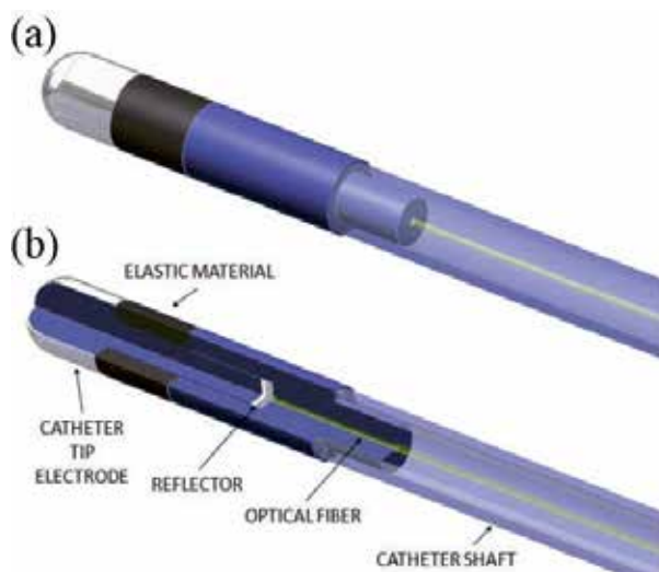
Figure 12. (a) Ablation catheter with force sensor. (b) Detailed view of this ablation catheter (Reference [29]).
