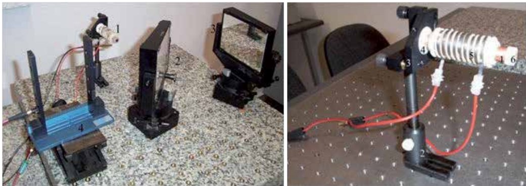
Figure 7. Schematic diagram of a free space Michelson interferometer for the measurement of thermal expansion coefficient for copper. 1, 2 – dielectric mirrors, 2 – beam splitter, 4 – observation plane (left), and detailed view on the investigated object (1) placed in a holder (2) with a micrometer screw (3), plastic isolation (4), heating coil, and a mirror in a mount (6) (right).
