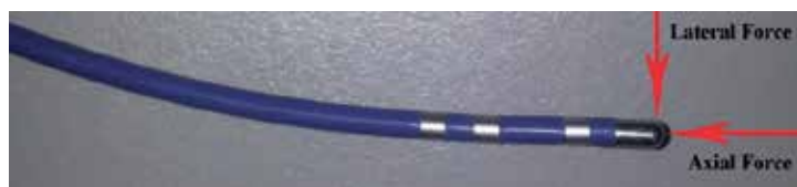
Figure 9. Axial and lateral force with respect to catheter's tip.
