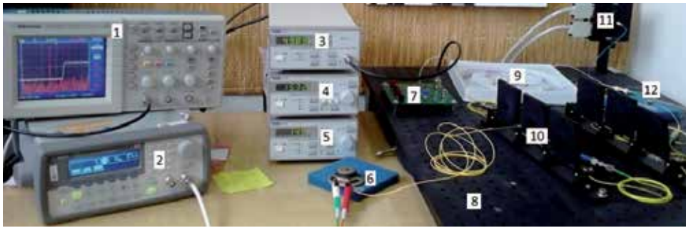
Figure 10. Practical arrangement of a fiber optic Michelson interferometer for the measurement of membrane vibration frequency. 1 – oscilloscope, 2 – waveform generator, 3 – electric amplifier, 4 – temperature controller, 5 – laser power controller, 6 – investigated object – a loudspeaker, 7 – photodiode, 8 – optical table, 9 – fiber coupler, 10 – polarizer, 11 – DFB laser in a special holder, 12 – pigtailed fiber mirror.
