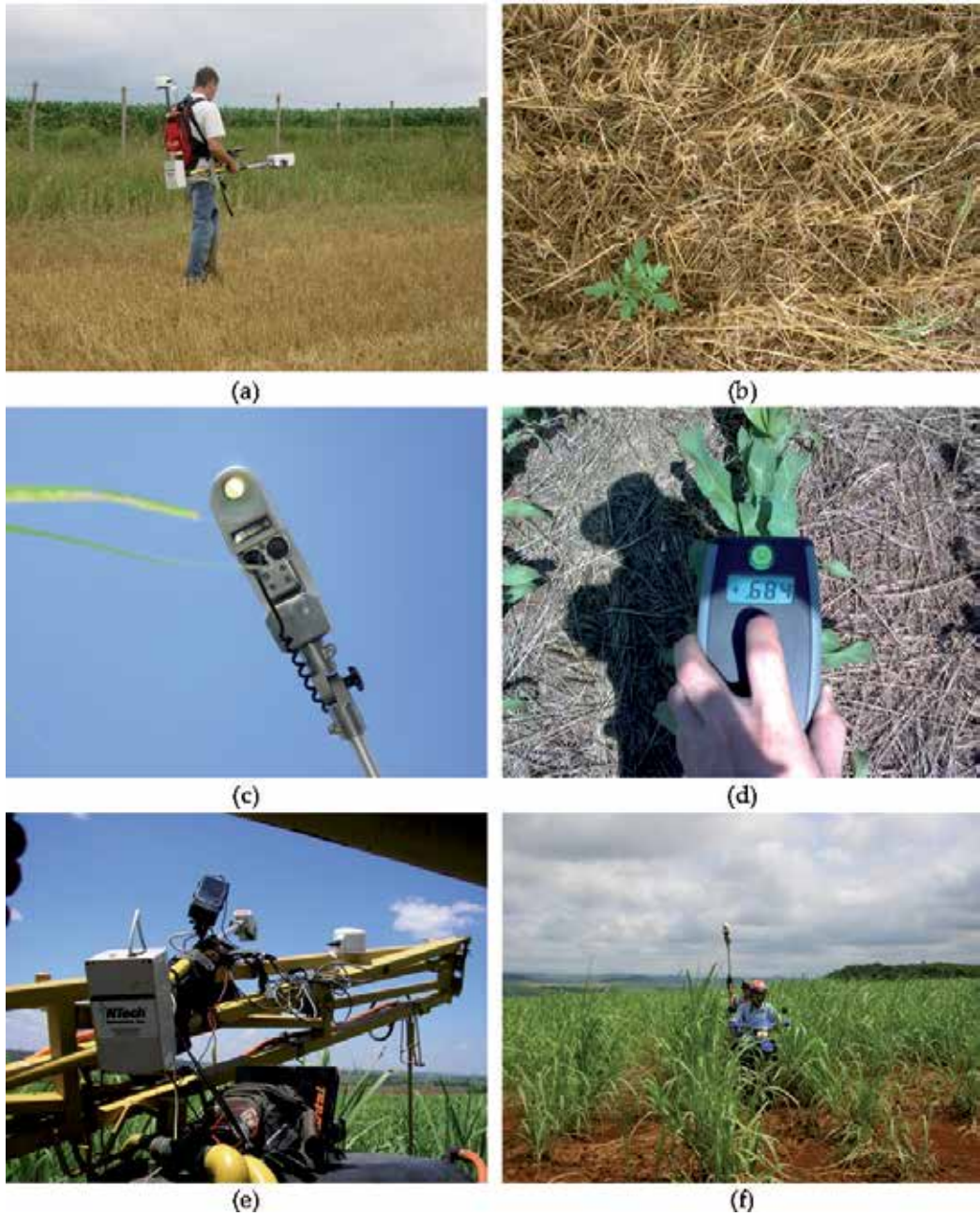
Figure 2. GreenSeeker sensor collecting NDVI values for weed (a) and (b); detailed pictures from GreenSeeker Hand Held (c) and Pocket Sensor (d); and GreenSeeker mounted on a sprayer (e) and on a motorcycle (f) collecting NDVI values in sugarcane.
