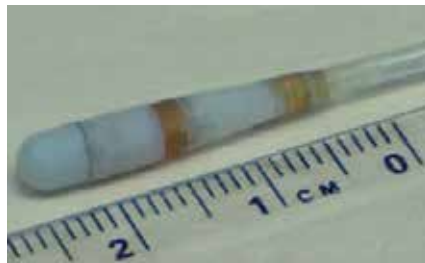
Figure 14. Ablation catheter with tri-axial force sensor
