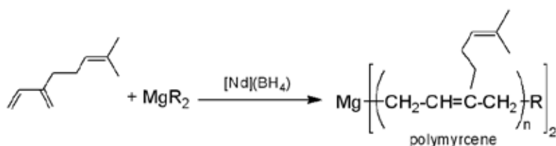
Scheme 16. Oligomerization of myrcene by CCTP with rare earth / magnesium system. [\text{Nd}](\text{BH}_4)_2 = \text{Nd}(\text{BH}_4)_3(\text{THF})_3 , \text{Cp}^*\text{Nd}(\text{BH}_4)_2(\text{THF})_2 , \text{MgR}_2 = \text{BEM} .
