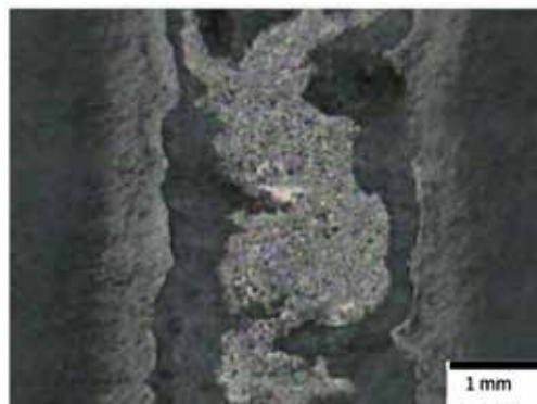
Figure 8. 32CrMoV12-28 steel alloyed with Si 3 N 4 powder, laser power 1.2 kW
