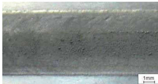
Figure 19. Surface layer of the MCMgAl9Zn1 alloy after WC powder feeding, laser power 2.0 kW, laser scan rate 0.5 m/min
