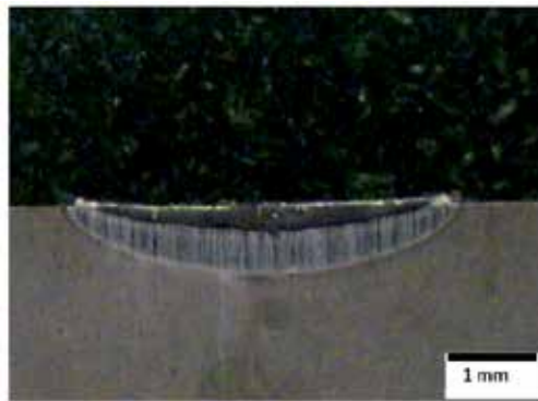
Figure 10. 32CrMoV12-28 steel alloyed with VC powder, laser power 1.2 kW
