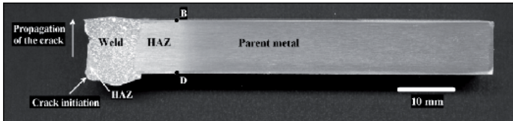
Figure 23. Typical macrograph of the fatigue failure on MIEA welds.
