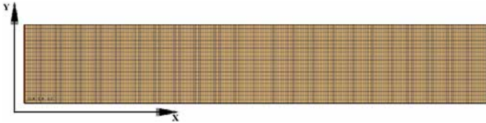
Figure 1. Computational domain and mesh of a generic cylindrical aquifer
