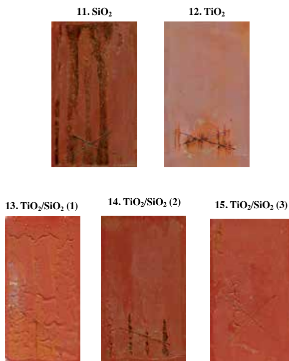
Figure 6. Photos of paint films of Group III after immersion in 3.5% NaCl after 28 days
