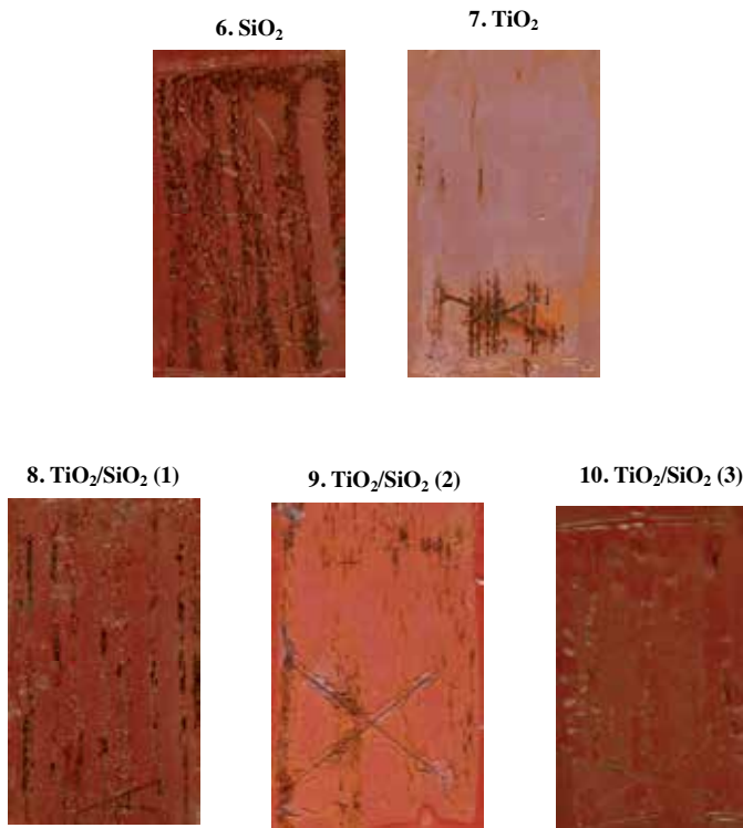
Figure 5. Photos of paint films of Group II after immersion in 3.5% NaCl after 28 days
