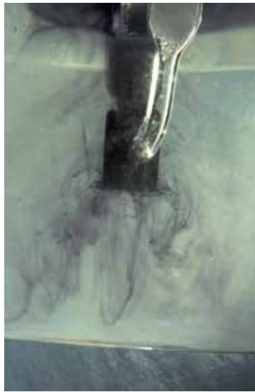
Figure 7. Iron-tannate precipitate forming on a steel plug in a solution with the same tannin concentration and pH as white oak. SCALE: The steel plug is approximately 9.5 mm in diameter.
