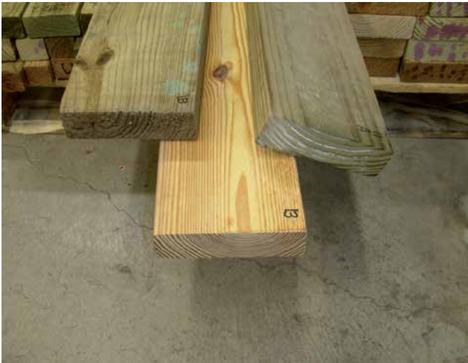
Figure 3. (From left to right) Wood treated with MCQ, DDAC, and ACQ. Cupric ions from the wood preservative cause the dark coloration of the wood. Excess copper has deposited on the MCQ (green splotches) and the ACQ (along the end grain) samples. SCALE: The boards are approximately 38 × 140 mm.
