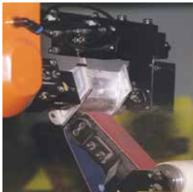
Fig. 17. Robot holding workpiece in contact with the polishing belt.
