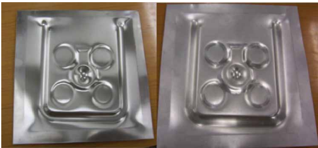
Fig. 18. Formed chair backs: AISI 304 (left) and DC04 (right).
