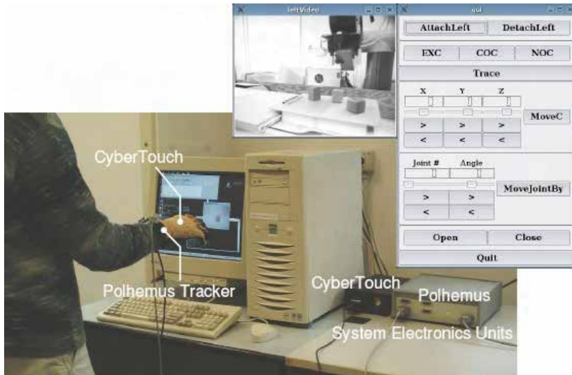
Fig. 10. An example of the client setup, and a snapshot of the GUI with a window displaying sensory information received from the remote site.
