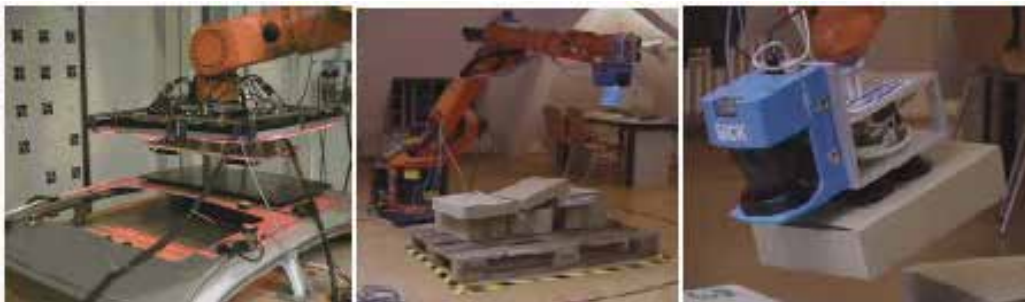
Fig. 10. (a) The sunroof fitting robot using four cameras in a closed loop control scheme and (b), (c) the depalletizing system during scanning and grasping
