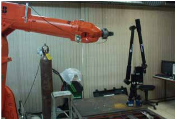
Fig. 6. Coordinate Measuring Arm - ITG ROMER and ABB IRB-2000 manipulator (University of Brasilia).
