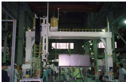
Fig. 9. General view of the welding robot equipment.
