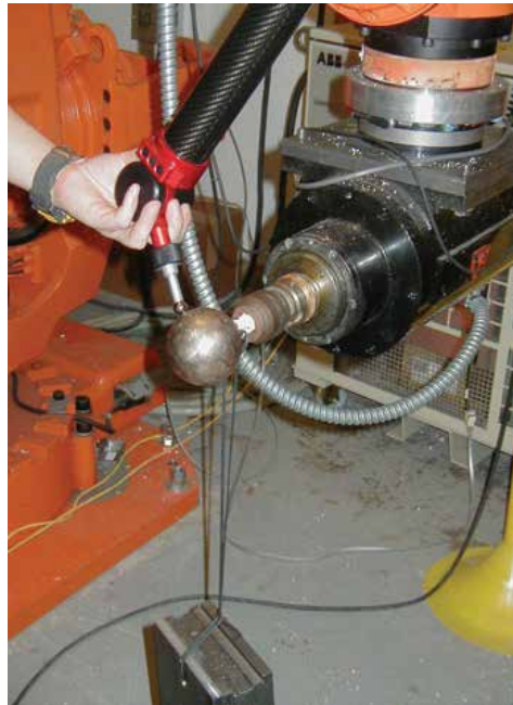
Fig. 15. Experiment Setup for robot stiffness measurement.
