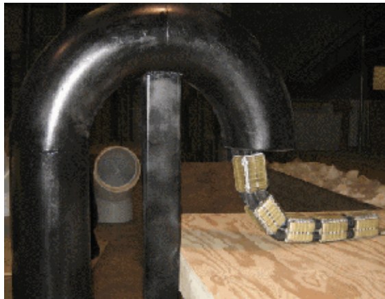
Fig. 1. The OmniTread Model OT-4 serpen-tine robot entering an “Inverted-‘J’” ventilation duct at SwRI†.
