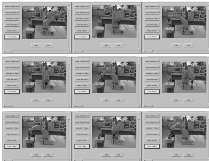
Fig. 10. Remote access to the hand-eye system; The remote user uses the telerobot system to manipulate the juice, fork, green cup and vitamin drink and put them to the tray mounted on the mobile platform.
