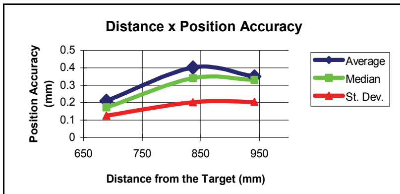
Fig. 10. Measurement system 3-D position accuracy versus the average distance from the camera focal point to the central point of the target.
