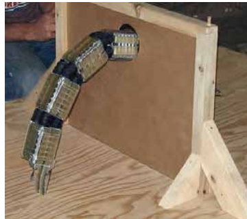
Fig. 6. OT-4 passes through a 10-cm (4") diameter hole, high above ground. Extendable "flipper tracks" in the distal segments allows the robot to straddle the hole without having to support its weight on the sharp edges of the hole in this test at SwRI.
