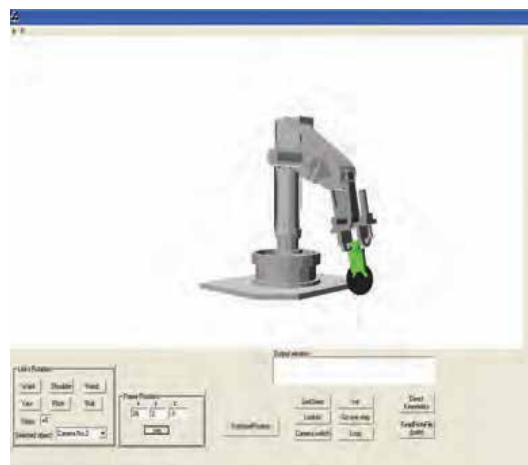
Fig. 11. The robot picture after reaching the end effector to target (view camera2).
