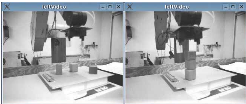
Fig. 13. A stacking experiment with the Puma 560 manipulator. The images are taken from the left eye of the stereo camera.
