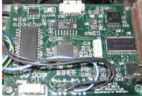
Fig. 19. Drive Motor Controller Board. This board generates the PWM signals for the off-the-shelf digital power amplifier for the OT-4 motor.
