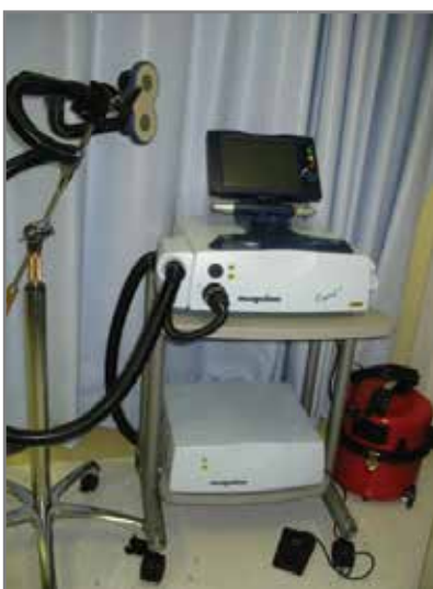
Fig. 4. Magstim super-rapid 2 TMS device at BNL that can deliver pulses reaching up to 100 Hz.
