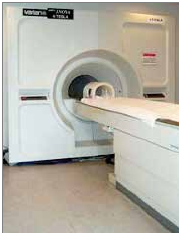
Fig. 2. 4 Tesla MRI Varian scanner at Brookhaven National Laboratory (BNL)
