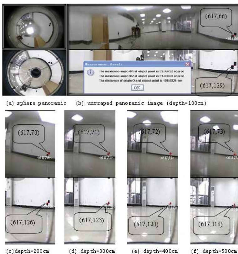
Fig. 17. Experiments for matching the object point and measuring the depth of object point
