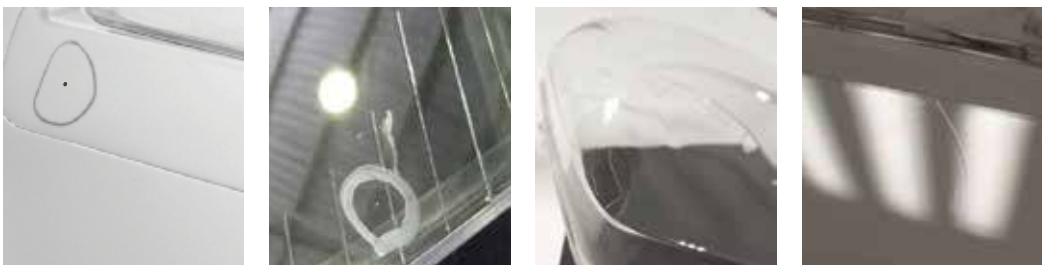
Fig. 2. Aesthetic defects. From left to right: punctual and opaque defect (a black point), punctual and transparent defect (a blister), lineal defect (a scratch) and surface defect (excesses of varnish).
