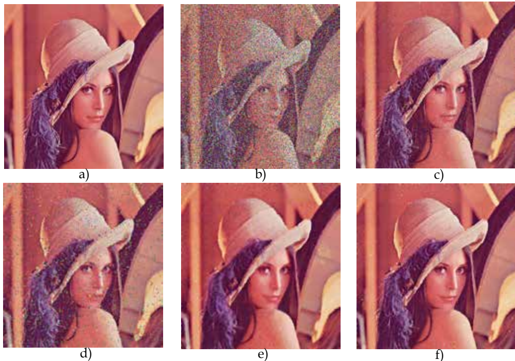
Fig. 5. Subjective visual qualities of restored colour image "Lena", (a) Original test image "Lena", (b) Input noisy image (with 20% of impulsive noise), (c) FASVM filtering image, (d) VMMKNN filtered image, (e) Proposed VMML filtering image (S,E,ND), and (f) Proposed VMML filtering image (S,E,D).
