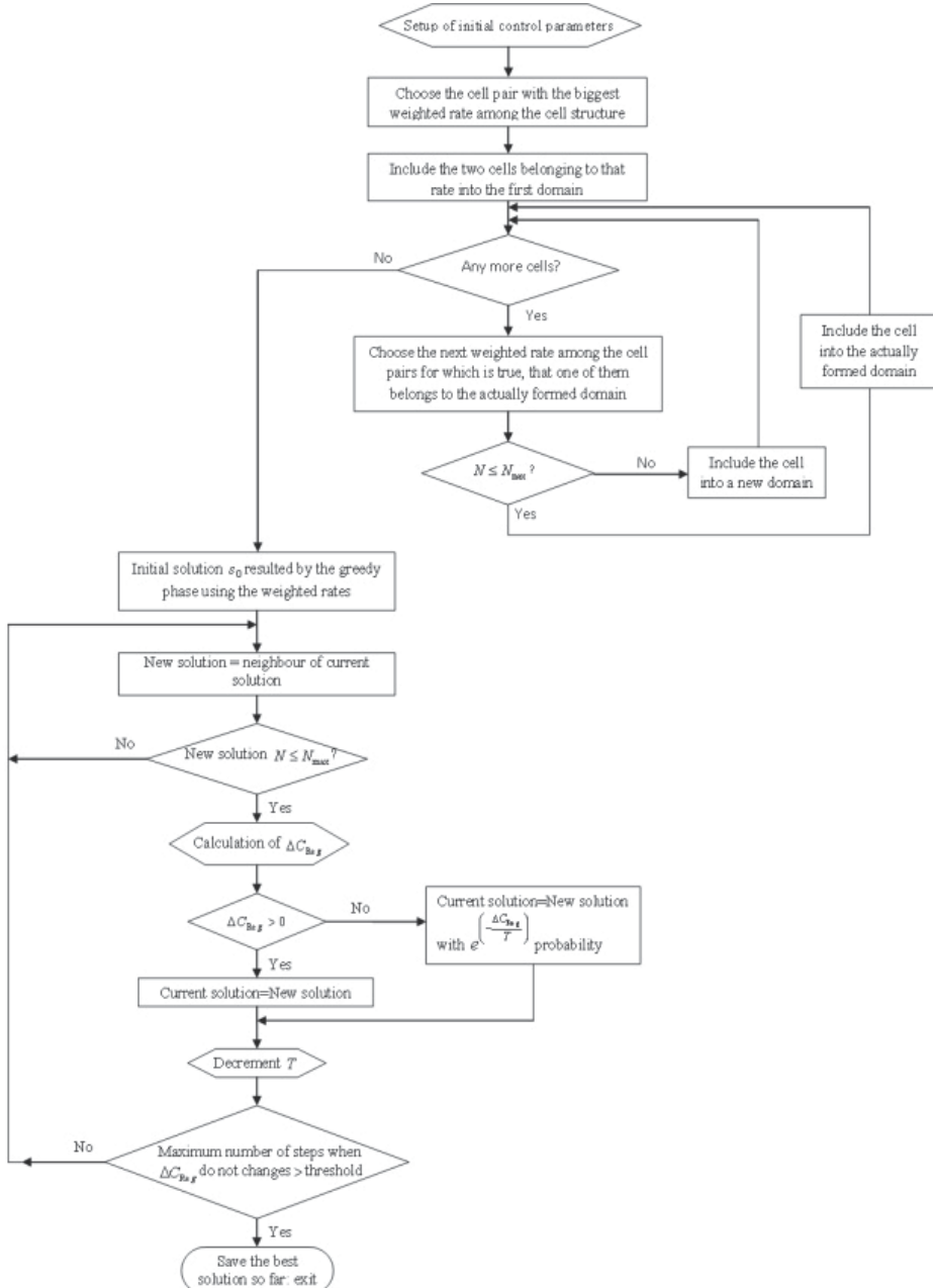
Fig. 1. The detailed flowchart of our proposed location privacy aware domain planning algorithm
