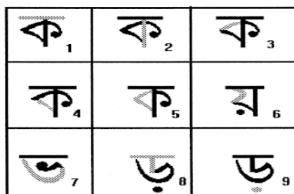
Fig. 8.1.4 Stroke features used for character recognition. (Shaded portions in the character represent the features)
