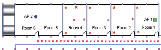
Fig. 8. Layout of the classrooms building with the location of the measurements points and APs
