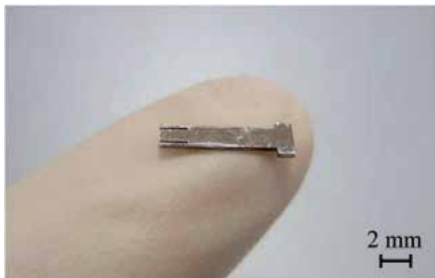
Figure 13. Fabricated and assembled single link part for the microarm
