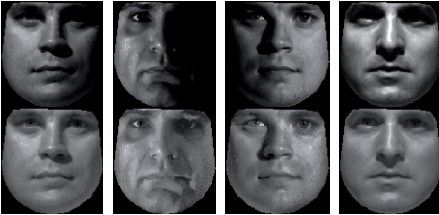
Fig. 2. Illumination normalization using histogram fitting: On the top the input images are given, and on the bottom the normalized images are shown.
