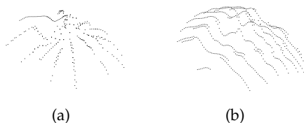
Fig. 4. Points on profile curves with curve parts under the same angle (a) or with the same x -value (b).
