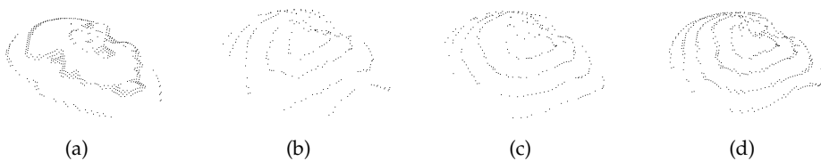
Fig. 3. Points lying on iso-depth curves (a), on iso-radius curves obtained by intersection with a cylinder (b) or with a sphere (c) and iso-geodesics with respect to the nose tip (d).
