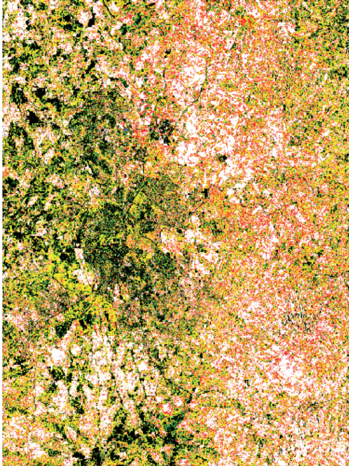
Figure 9. Result of combining the classification results of the two amplitude images from Figure 8 according to Table 1, where: L – black, C – blue, ML – green, M – yellow, MH – red, H – white.
