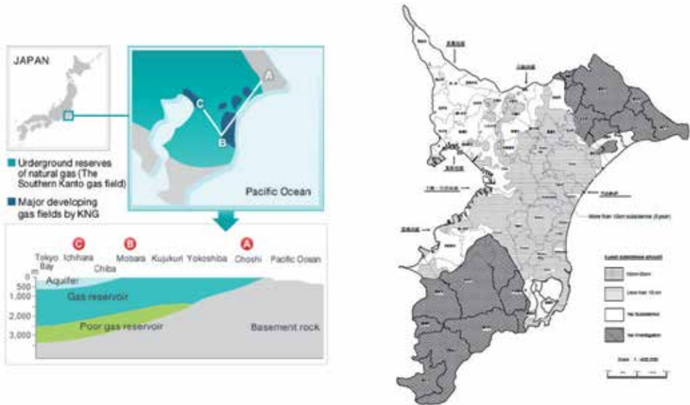
Figure 13. Southern Kanto gas field, Kanto Natural Gas Development Co Ltd. [19] (on the left); known 5-years displacement in the region of Togane, eastern part of the same area [20] (on the right).
