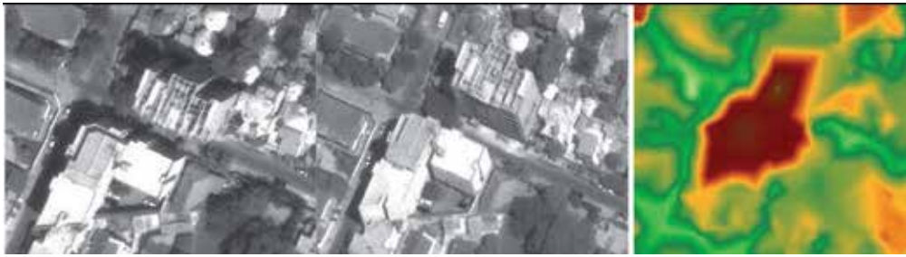
Figure 15. Example of corridor occlusion due to tall buildings; (a) and (b): stereo images; (c) resulting DEM (Dakar).
