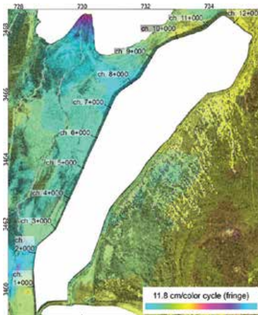
Figure 10. ALOS palsar filtered interferogram showing ground deformations recorded from 2008-04-01 to 2008-05-17 (46 days). The short baseline of 41 m leads to an altitude of ambiguity of 1551 m. The image image is therefore a "true" differential interferogram. Because of L-band, some deformation fields appear clearer than with C-band in the most active zones such as the delta of wadi Araba.
