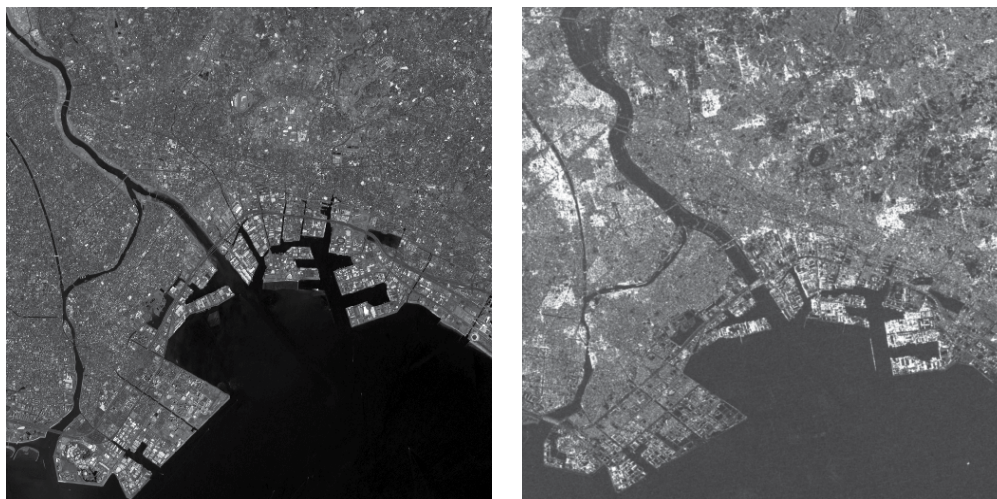
Fig. 4. ASTER (left) and PALSAR (right) images of Tokyo bay, Japan with 512x512 pixels
