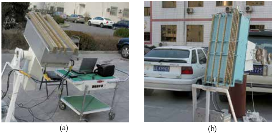
Fig. 8. One dimensional interferometric radiometers built by CSSAR
