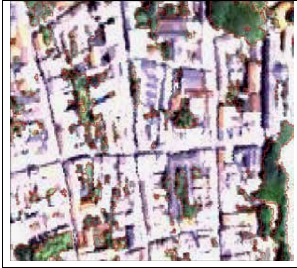
Fig. 4. Sample output of the automated identification and contouring process of buildings and vegetation, done on 56-channel AISA hyperspectral VNIR data by use of a patented method, mutated by burn scar analysis (Ferrucci & Hirn, 2005). In these pixels, LiDAR elevation measurement are expected to be precise within the error estimate ( \pm 0.15\text{m} averaged over buildings and bare soils).
