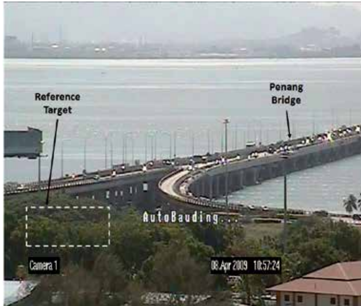
Fig. 6. The reference target of green vegetation captured by the internet surveillance camera
