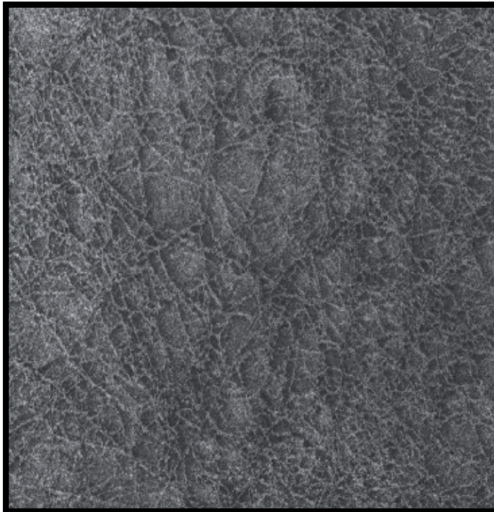
Fig. 3. Reduced back-scattering in areas bordering pressure ridges on a RadarSAT 1 image of a first year sea ice.
