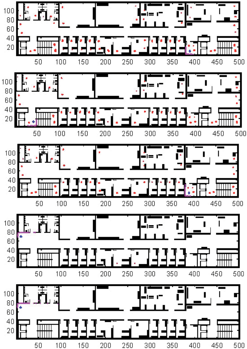
Fig. 9. Convergence process along 5 successive perception-motion cycles where the robot turns 10^\circ clockwise after each perception cycle.
