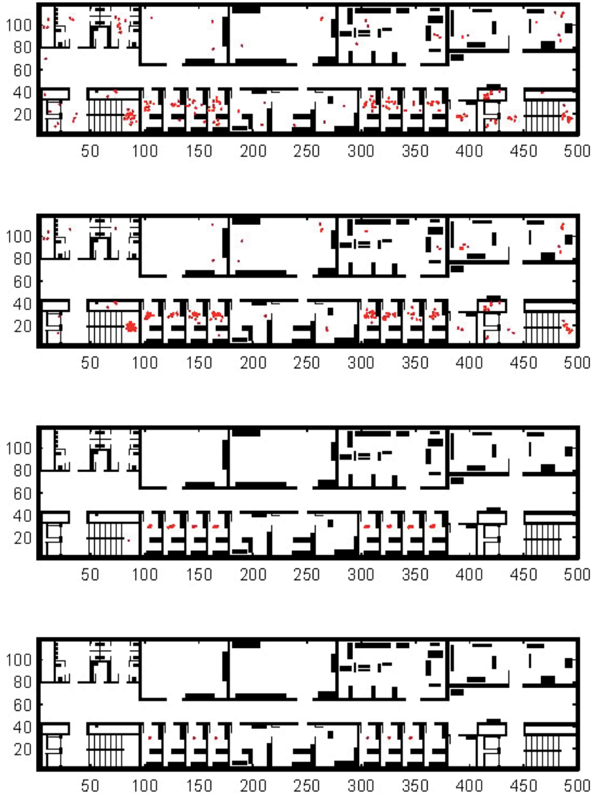
Fig. 2. Premature hypothesis elimination, initial pose (105, 30, 270), 200 elements in population and \sigma of 3% of the measured signal.
