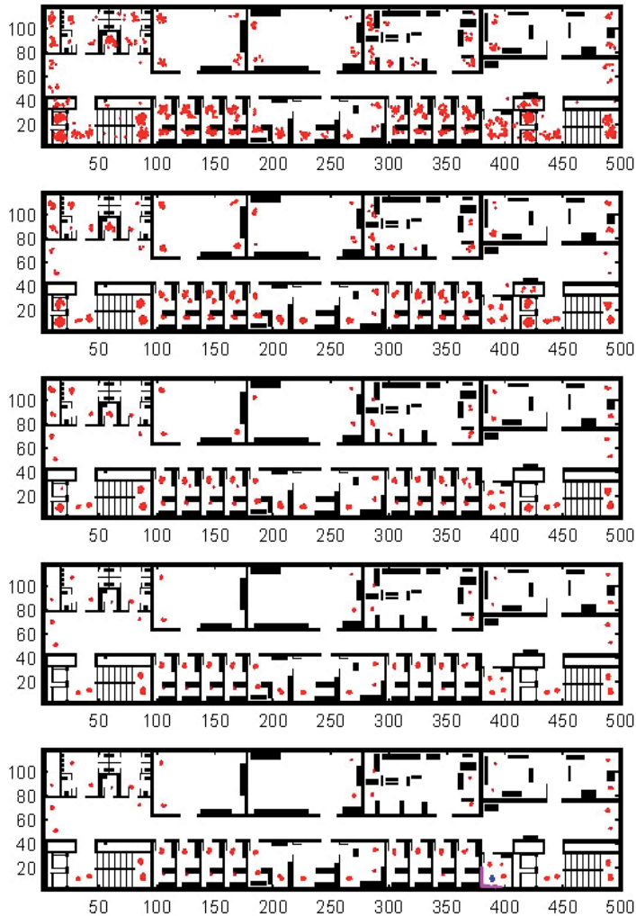
Fig. 8. Convergence process for the worst case pose ( 100, 200, 300, 400, 420) of the first perception cycle.
