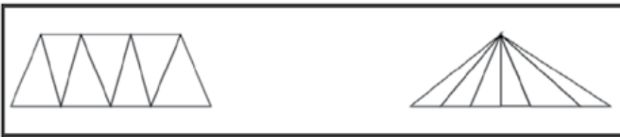
Fig. 3. Triangle strips and triangle fans can reduce the number of redundant points.
