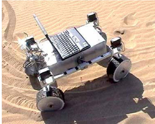
Fig. 1. Significant wheel slip and sinkage of the rover Dune, constructed at the University of Salento
