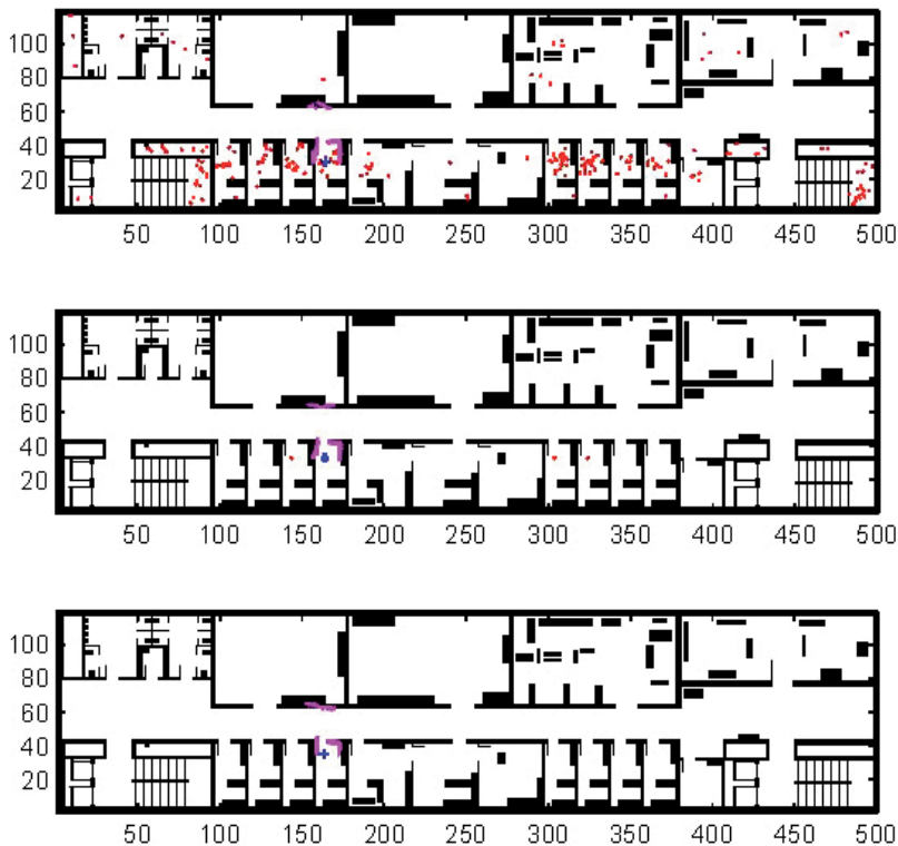
Fig. 3. Premature hypothesis elimination, starting pose (305, 30, 270), 200 elements in population and \sigma of 3% of the measured signal, motion +2.5 cells per cycle in y direction.
