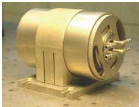
Faraday isolator with slab magneto-optical elements
