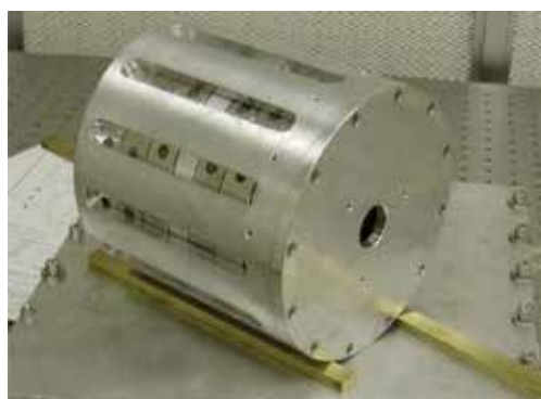
Faraday isolator for vacuum application
