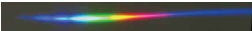
Fig. 14. Photo of the spectrally resolved filamentation output in the self-compression regime. Concerning the CEP stability of the filamentation output, several femtosecond filamentation experiments performed at various center wavelengths (Hauri et al., 2004, 2007) have clearly demonstrated that the filamentation process preserves the CEP stability of the input pulses. Therefore, we are convinced that the filamentation process does not degrade the CEP stability of the OPCPA input pulses in our experiment. Nevertheless, in order to quantify the quality of CEP stability, we are planning (i) to perform inline f -to- 2f interferometry to the OPCPA output of stages 3 and 4, (ii) quantify possible differential CEP drifts caused in the individual amplification stages 3 and 4 using a TADPOLE-type technique, (iii) and finally perform f -to- 3f interferometry (since a sizable third harmonic is generated inside the filament) to the filamentation output.
