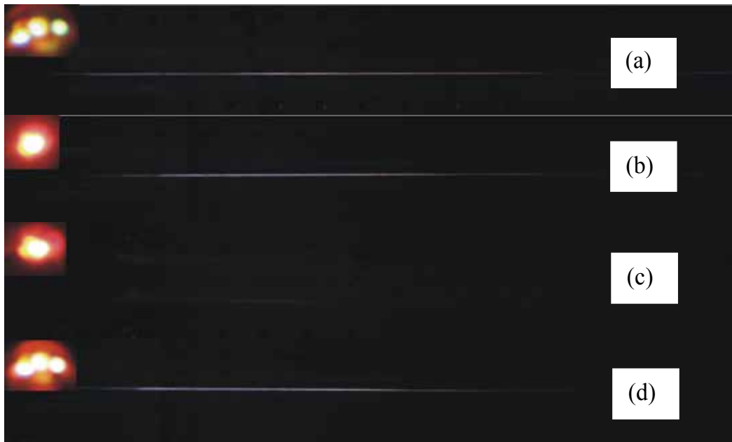
Fig. 14. Filament pattern at temperature of (a) 25 °C; (b) 200 °C; (c) 300 °C; (d) 25 °C. The inserted pattern in every picture is the output beam profile.
