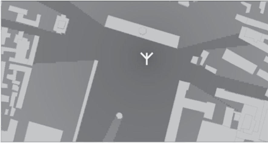
Fig. 6. Top view of the discrete line-of-sight region (dark grey) with the source point in the center (white cross). Building interior is shown in light grey.
