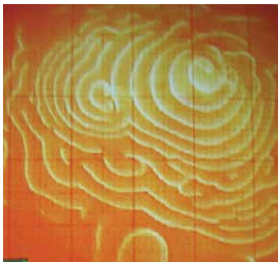
Fig. 6. Open fronts and spiral fragments in propagating BZ waves in gels made with heavy water.
