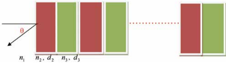
Fig. 1. Stack of 1 D MDPC ,where n_2 is the refractive index of the metal, d_2 is the thickness of the metal , n_3 is the refractive index of the dielectric material and d_3 is the thickness of the dielectric material.
