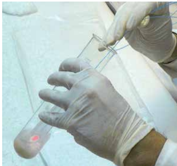
Fig. 1. Photograph of the special lucite test tube with copper mesh bottom (not seen) placed inside a standard glass laboratory test tube during in vitro fragmentation of an artificial infected kidney stone with a laser lithotripter.
