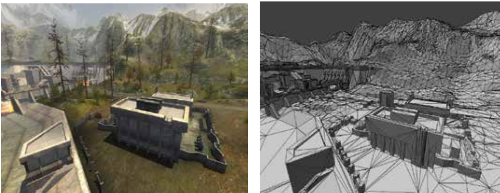
Figure 2. Boundary representation of C-Space for an outdoor environment with buildings
