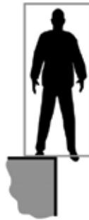
Figure 4. A robot partly standing over a ledge while the bounding box rests upon the edge
