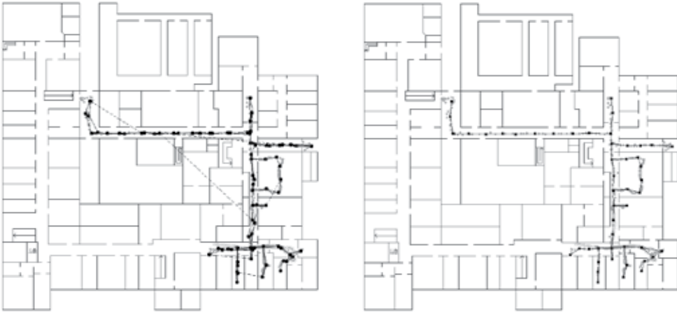
Figures 11 (left) and 12 (right). Left: topological loop closing, accepted hypotheses are shown in thick black lines, rejected in dashed thin black lines. Right: the resulting topological map, locations of the place prototypes with interconnections
