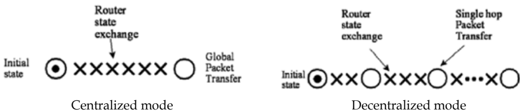
Figure 12. centralized and decentralized modes in a discrete HPF paradigm
