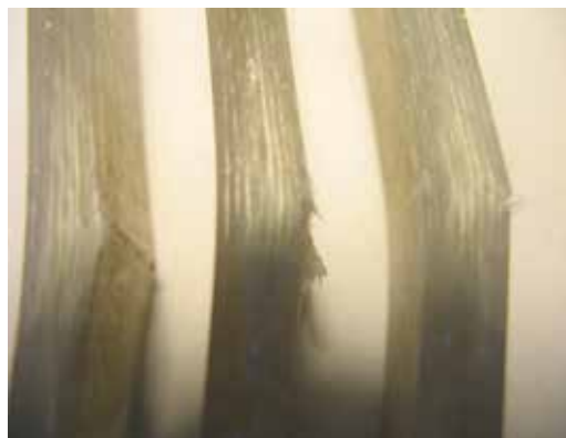
Fig. 33. Failure area of some specimens reinforced only with E-glass fibres, after flexural test
