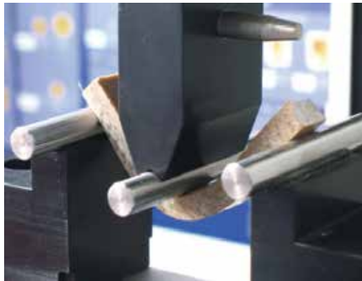
Fig. 5. Specimen made of E-glass EWR145 / oak wood flour / polyester Colpoly 7233 during flexural test
