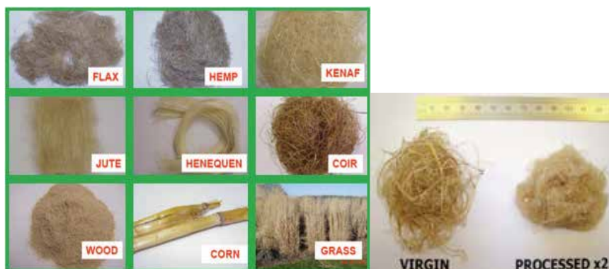
Fig. 4. (a) Some natural fibre, (b) Unprocessed and Processed hemp fibres (source: University of Exeter)
