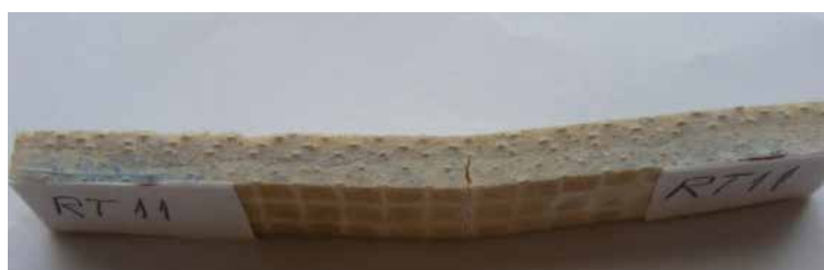
Fig. 36. Photo of the specimen surface made of E-glass EWR145 / fir wood flour / polyester Colpoly 7233 after immersion in water (5612 hours)
