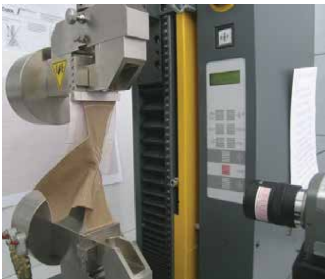
Fig. 4. The way of sample mounting in the tensile machine jaws for the tearing zone registration Source: own
