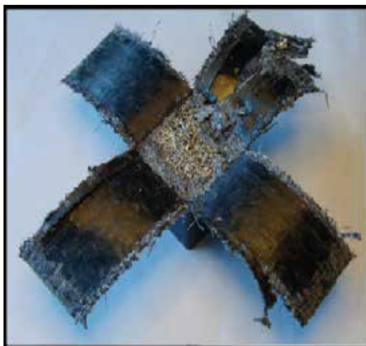
Fig. 16. Crush pattern of foam-filled composite crash box
