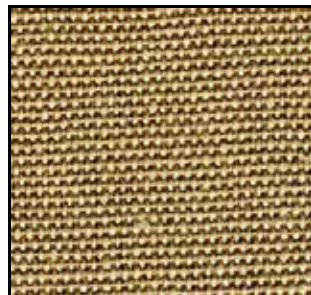
Fig. 15. Examples of plain woven flax yarns. H-181 100% Hemp Canvas weave 18oz/sq yd Wide 59" 5N/2 x 8N/2 x23x21. Source: dongpinghemp.com
