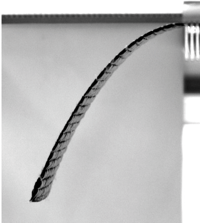
Fig. 10. Cantilever bending test
