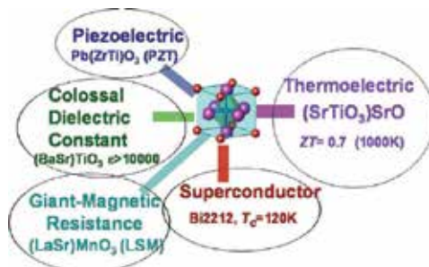
Fig. 2. As Perovskite-structure based materials are record holders in many solid-state properties, they might become so in thermoelectrics too.
