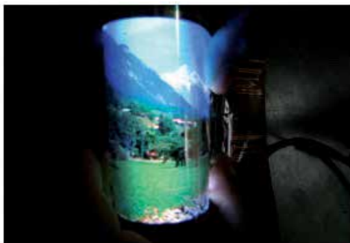
Fig. 28. 6.5" flexible AMOLED display by Samsung. ufigure LOGICAL ISSUES FOR SMALL-SIZED MOBILE OLEDD
