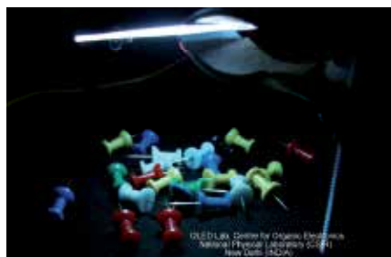
Fig. 2. 1"x1" proto type of a multilayer phosphorescent efficient WOLED developed at National Physical Laboratory, New Delhi, India
