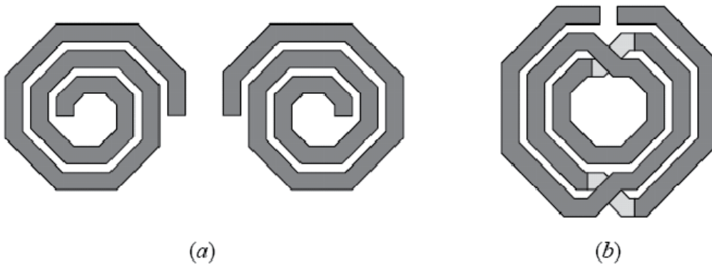
Fig. 13. A pair of single-ended inductors (a) and a differential inductor (b) with similar total inductance [4].
