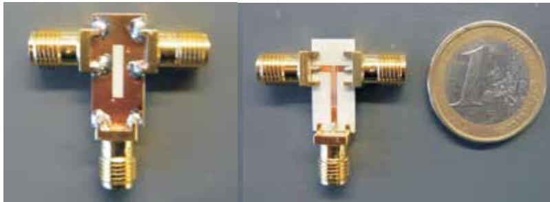
(a) Picture of implemented power splitter.
