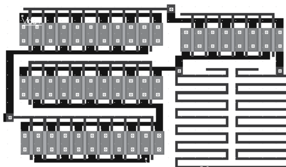
Fig. 56. Active inductor layout
