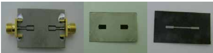
Fig. 6. Photograph of the fabricated UWB filter.
