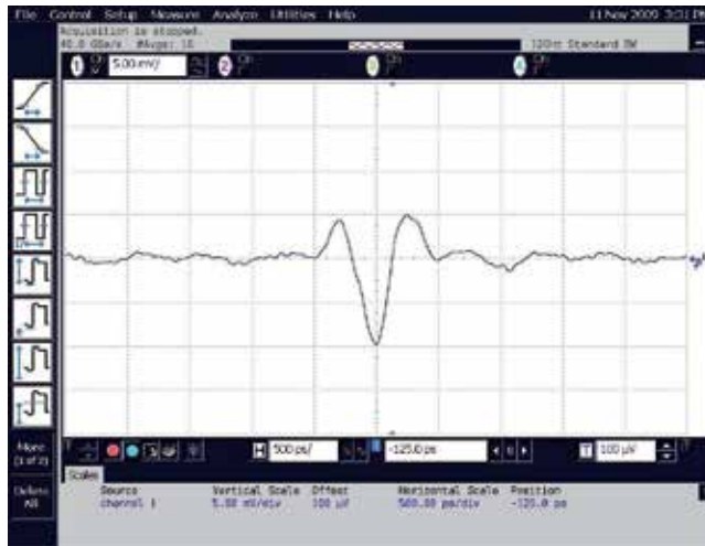
Fig. 7. The measured Gaussian doublet at the output of the passive UMZI system
