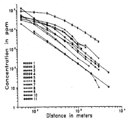
Fig. 14. EU Benchmark exercise to investigate uncertainty limits in risk assessment. Calculated ammonia concentration as a function distance 15 minutes after a  $NH_3$  liquid release, adopting different gas dispersion models (reproduced after Amendola et al., 1992).
