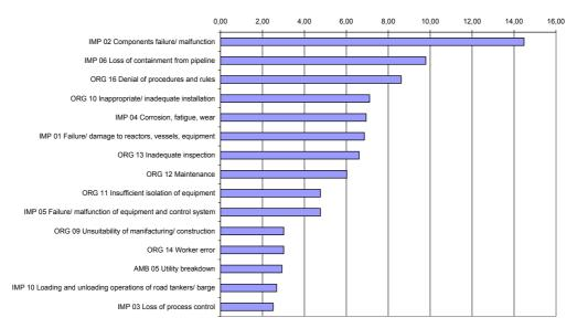
Fig. 11. Top fifteen immediate causes of near-misses (percentage of the entire number of entries) recorded in a downstream oil company over an eight-year period.
