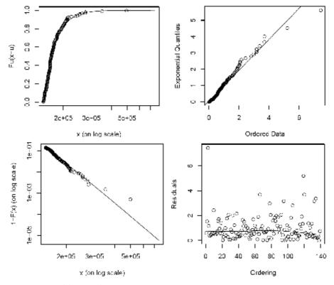
Fig. 9. Goodness of fit tests for GPD with estimated parameters  $\beta = 28.027,00$  and  $\xi = -0,0781$ .
