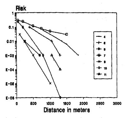
Fig. 15. Benchmark exercise to investigate uncertainty limits in risk assessment. Calculated individual risk as a function distance, after a  $NH_3$  liquid release scenario(reproduced after Amendola et al., 1992).
