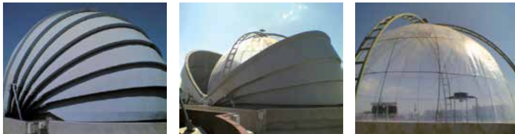
Fig. 1. EUPHORE Photoreactor: closed (left side of the figure), while opening (middle of the figure), and opened to sunlight (right side of the figure).
