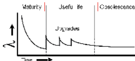
Fig. 14. Typical Bath-Tub curve for software (where \lambda is the failure rate).
