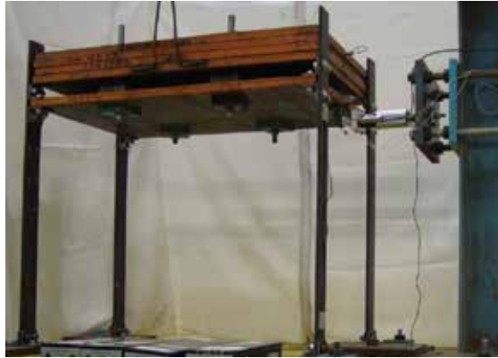
Fig. 11. Experimental setup for random vibration testing of self-sensing MR damper
