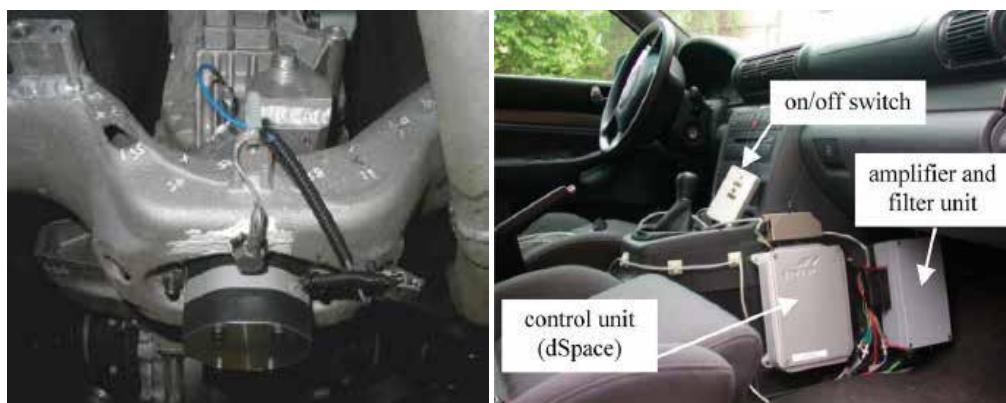
Fig. 8. Location of the AVC components in the test vehicle.
