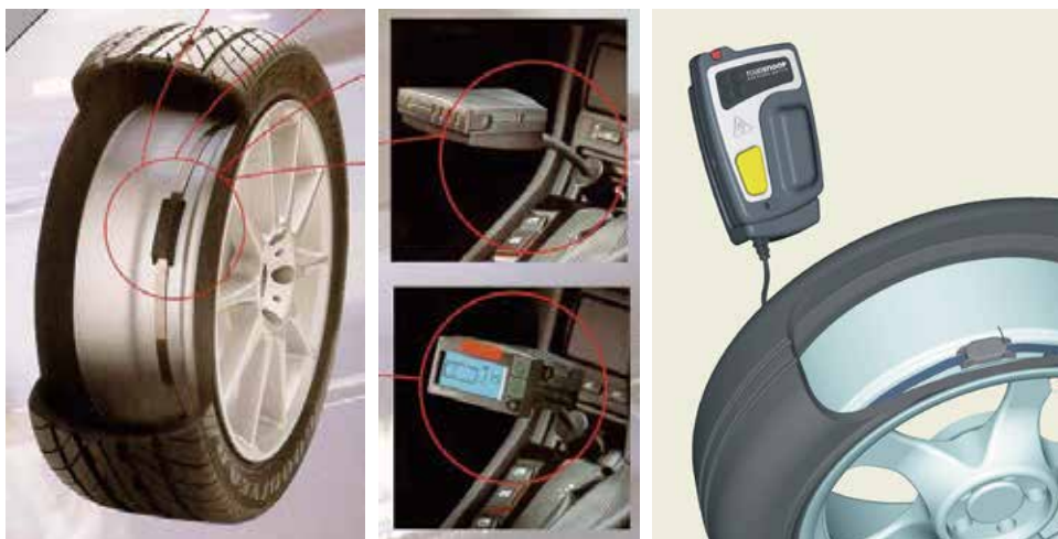
Fig. 3. SmarTire's TPMS product (Left) & RoadSnoop's Pressure Watch (Right)
