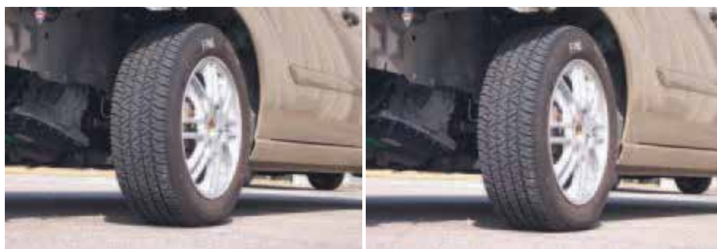
Fig. 1. A fully inflated tire (left) and one with only 70% pressure (right) (David, 2004)
