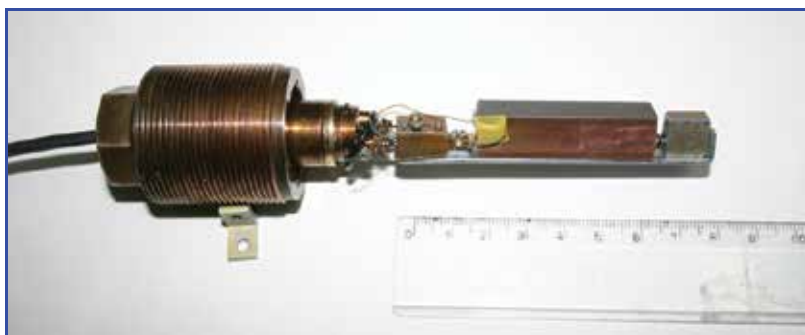
Fig. 4. Love wave waveguide (Cu surface layer on a steel substrate) connected to the high-pressure lead-through (on the left).
