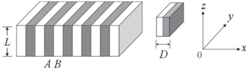
Fig. 1. 1D periodic composite plate consisting of alternate A and B strips.
