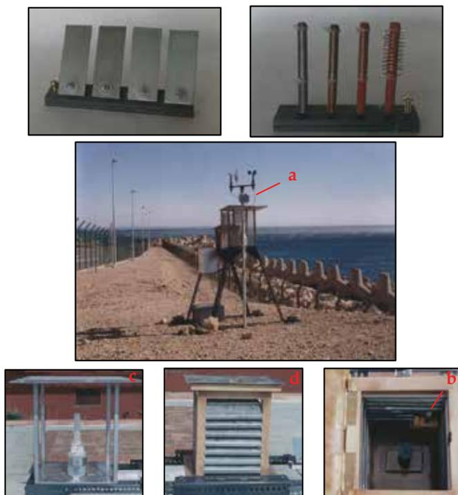
Fig. 3. View of a corrosion station (and corrosion samples) equipped with devices for recording meteorological (wind speed and direction (a), temperature and relative humidity (b) and pollution (salinity (c) and SO<sub>2</sub> (d)) parameters
