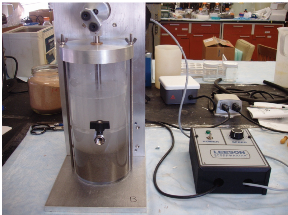
Fig. 1. Shaker for simulating erosion.
