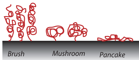
Fig. 1. Possible polymer conformations, depending on quality of solvent, polymer degree of ionization and grafting distance.
