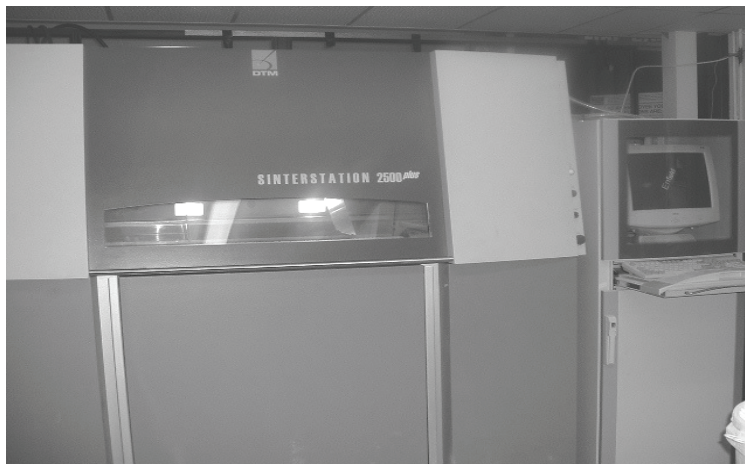
Fig. 4. The SLS Sintersation 2000 apparatus (Courtesy of CRDM)
