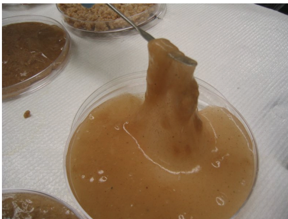
Fig. 11. Adhesive product of sand coated with guar gum cross-linked by borax.
