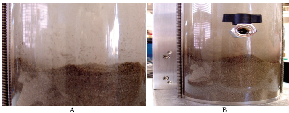
Fig. 17. Resuspension of organoclay (PM-199) leading to cloudiness (A) and surface suspension (B).
