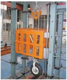
Fig. 7. Landing gear experiment platform
