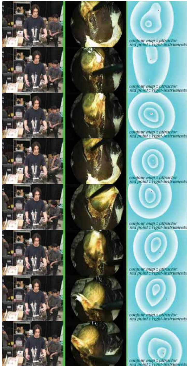
Fig. 6. View of an in vitro experiment (laparoscopic cholecystectomy) using a swine liver with a gallbladder (2/6). (left) a surgeon and the laparoscope robot P-arm, (mid) image from the laparoscope, (right) visualization of attractors as the contour map on the image plane.
