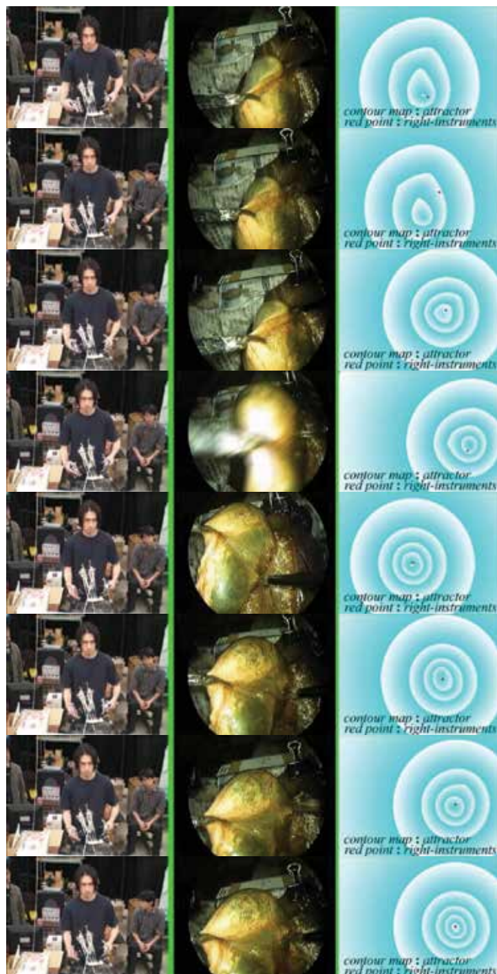
Fig. 9. View of an in vitro experiment (laparoscopic cholecystectomy) using a swine liver with a gallbladder (5/6). (left) a surgeon and the laparoscope robot P-arm, (mid) image from the laparoscope, (right) visualization of attractors as the contour map on the image plane.
