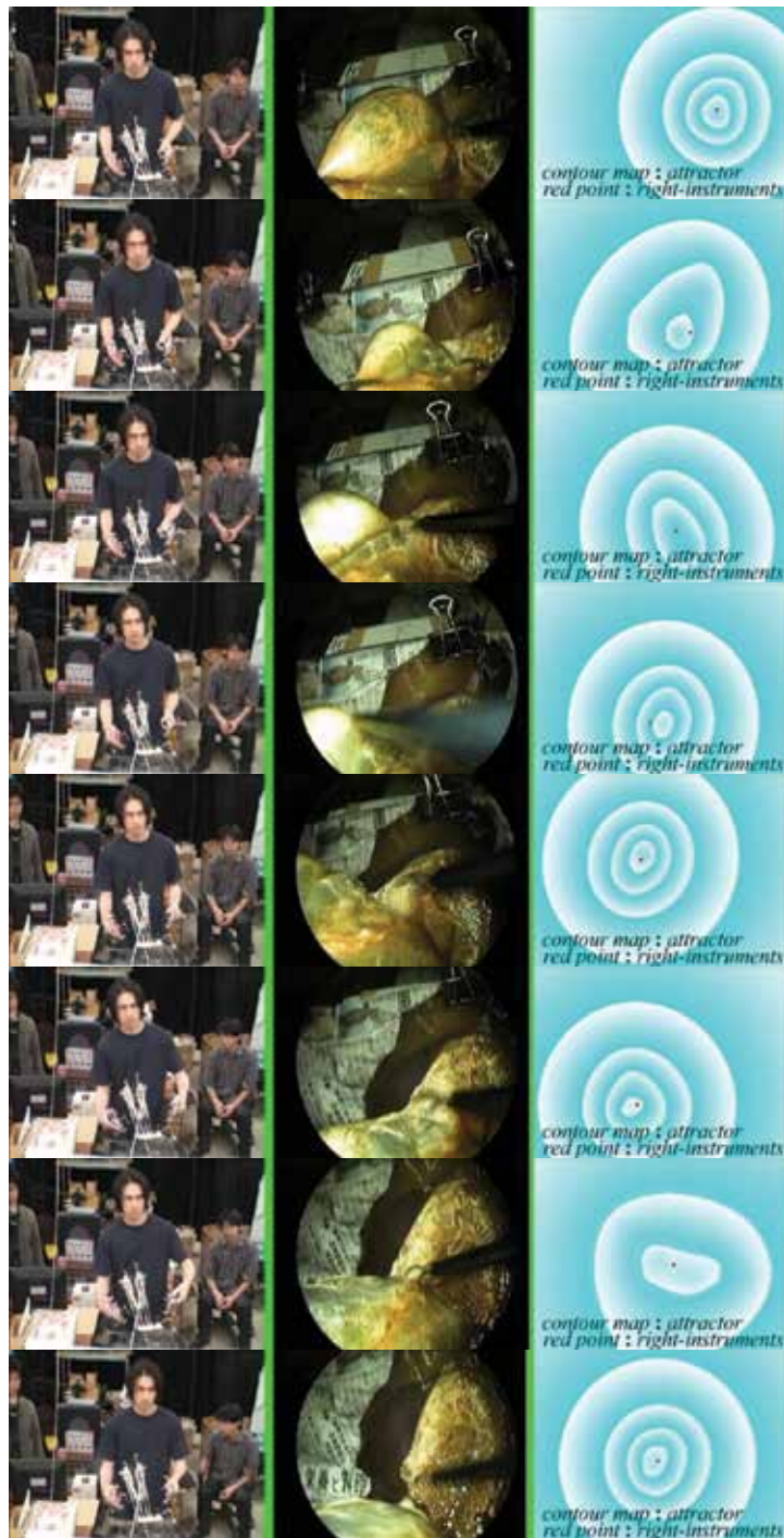
Fig. 10. View of an in vitro experiment (laparoscopic cholecystectomy) using a swine liver with a gallbladder (6/6). (left) a surgeon and the laparoscope robot P-arm, (mid) image from the laparoscope, (right) visualization of attractors as the contour map on the image plane.
