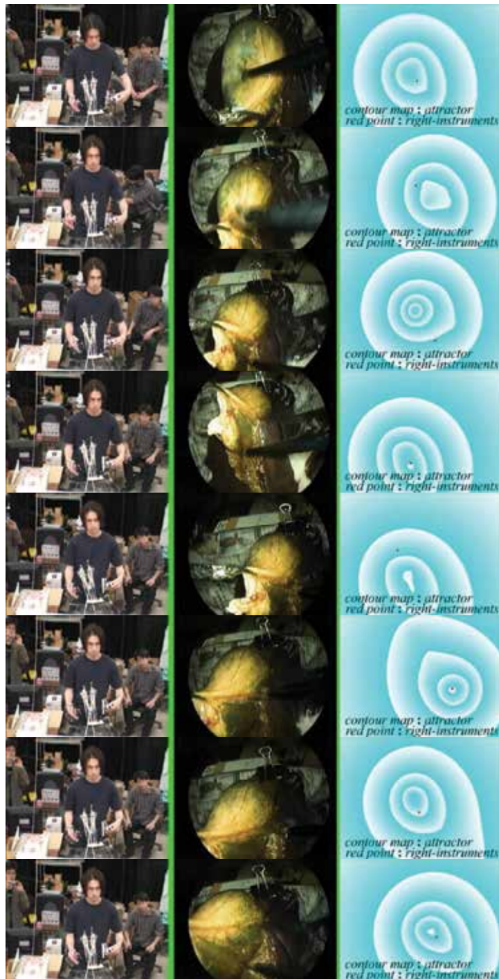
Fig. 7. View of an in vitro experiment (laparoscopic cholecystectomy) using a swine liver with a gallbladder (3/6). (left) a surgeon and the laparoscope robot P-arm, (mid) image from the laparoscope, (right) visualization of attractors as the contour map on the image plane.
