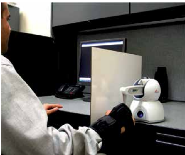
Fig. 5. The subject grasps the end-effector of the PHANTOM TM Omni and rotate his hand about his elbow.
