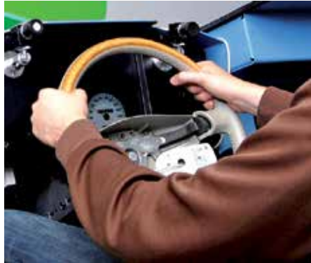
Fig. 3. A close-up of a subject holding the steering wheel, which could be perturbed or which could provide haptic guidance. The human reaction torque T_c and the resulting angular rotations X_c were measured.
