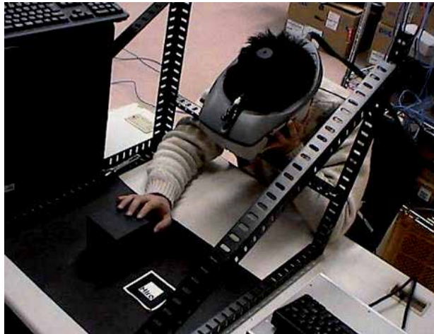
Fig. 9. Experimental of Subjective Evaluation of Sharpness. The subject maintains his viewpoint while putting his jaw at a predefined position to preserve geometric and photometric consistency between the real and virtual information.
