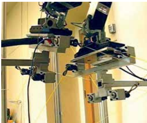
Fig. 10. Feet of the Kondo KHR-1HV on the scaled version of the CDLI
