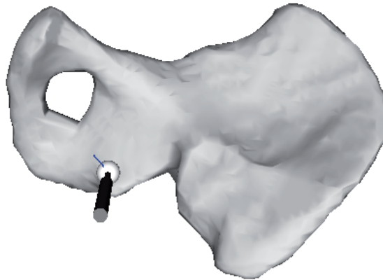
Fig. 12. A burr-tool receiving force-feedback from a polygonized pelvis model where the force (direction and strength) is displayed with a blue line
