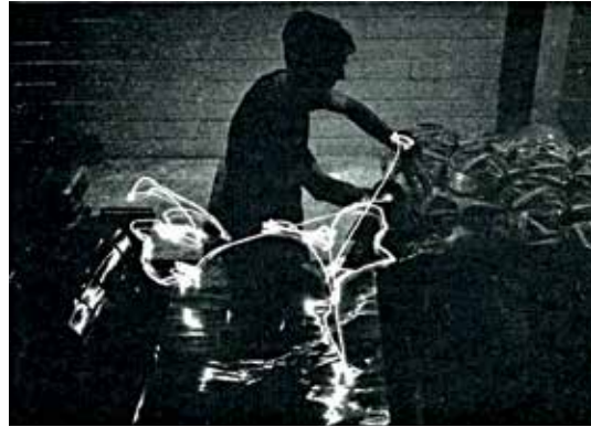
(a) Therblig Symbols (b) Chronocyclegraph Fig. 1. Gilbreth's Time and Motion Study (courtesy of Johnson & Ogilvie, 1972)
