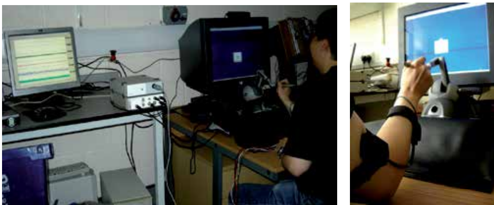
Fig. 11. Investigating haptic influence on motor control through biometric data logging. The experimental setup is shown on the left. The right image shows the goniometer attached to the subject's arm.
