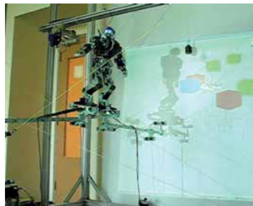
Fig. 11. Full view of the scaled version of the CDLI showing the platforms, the cables and the Virtual Reality screen displaying the scene
