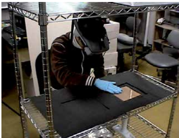
Fig. 5. An Experimental Scene of Evaluation. We use a glove that deadens the haptic sensation to maintain balance of haptic and visual stimuli.
