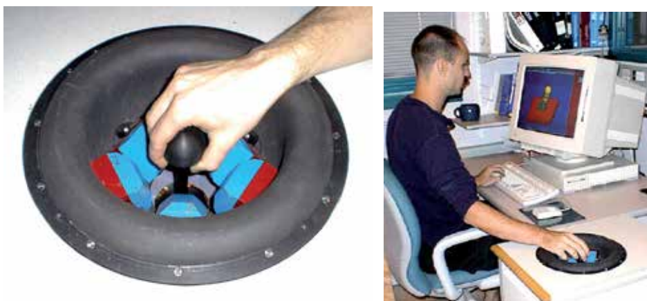
Fig. 3. Carnegie Mellon University Prototype (a) Levitated Handle Grasped by User, (b) Interaction with Simulated Environment
