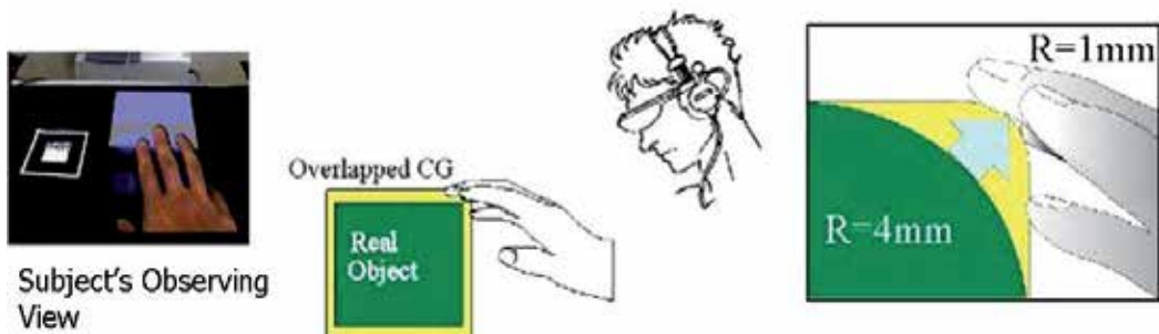
Fig. 8. Overview of Subjective Evaluation of Sharpness Sensation. We conducted an experimental survey to investigate whether an edge is perceived sharper than its actual curvature (4 mm) by overlapping a sharper appearance (1 mm) on the surface.
