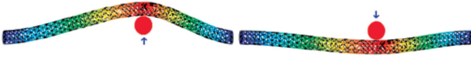
Fig. 4. Two deformations of the object for the identical position of the probe (depicted by the filled red circle) showing the non-flatness of the probe interaction model. On the left, the probe comes from the space below the deformable body, on the right it comes from the space above the body (the directions are depicted by the blue arrows).
