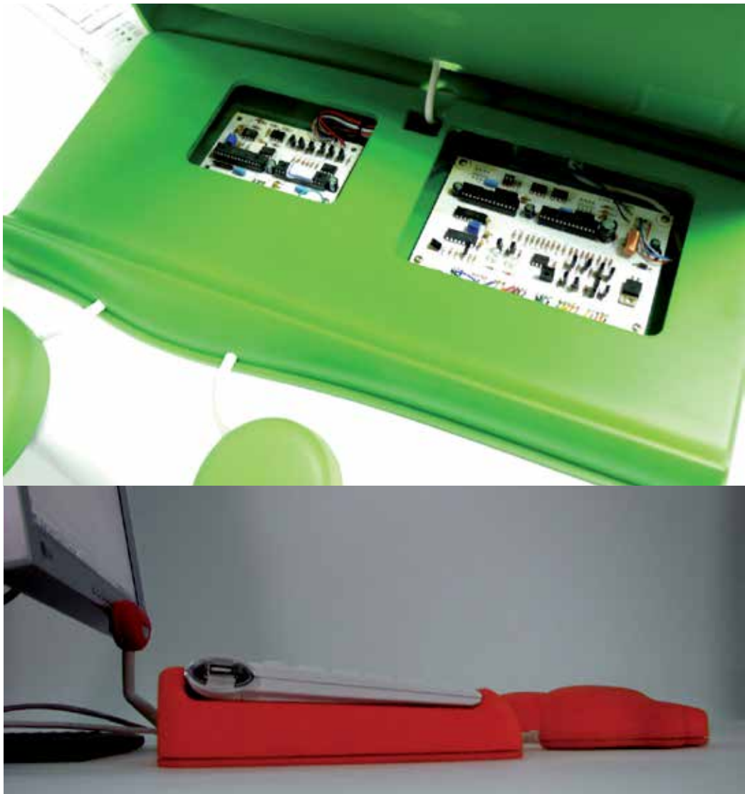
Fig. 10. Controller circuits underneath the keyboard base
