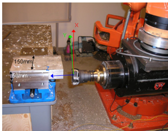
Fig. 6. Robotic end milling process setup
