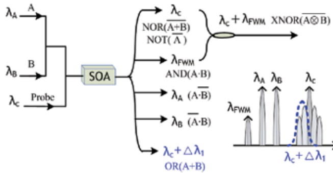
Fig. 17. Illustration of operational principle of the configurable logic gates
