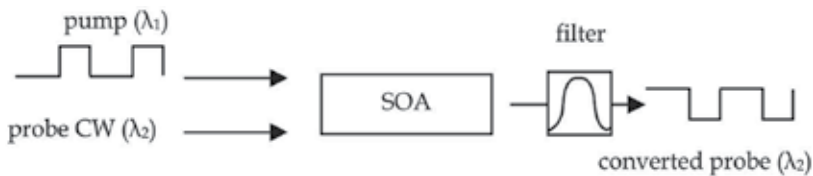
Fig. 6. Cross gain modulation (XGM) in a SOA.
