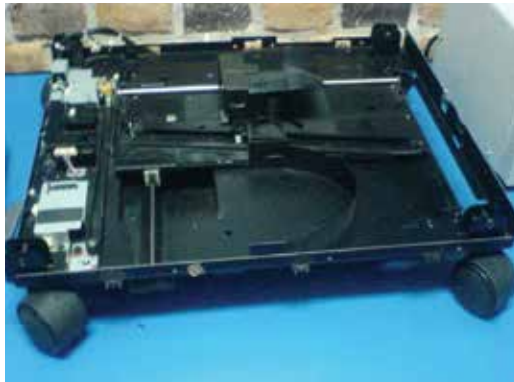
Fig. 24. XY table used as irradiance meter.
