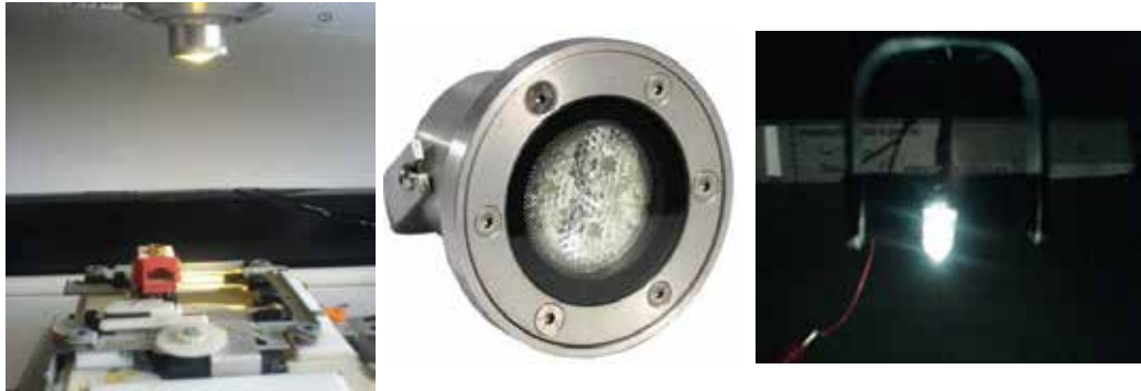
Fig. 18. (a) Dirigible X-lamp LED IL51, as a sample and the XY table. (b) Lamp IL/1 L3 (with a 3 LED array; and (c) single white LED
